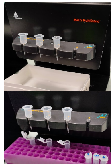
Figure 53 : Pictures to show how to use the \mu\text{MACS} columns in the magnetic stand. The top picture is when the columns are washed. The bottom picture is when the flowthrough is collected.
