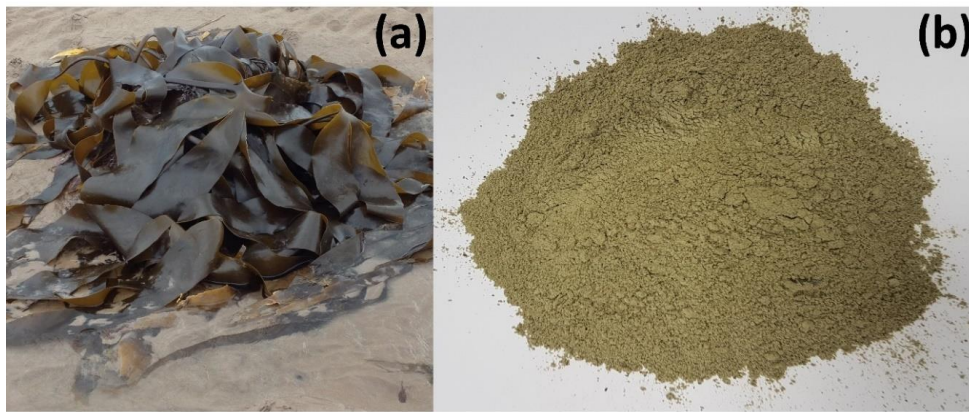
Figure 3-10 (a) Stranded Laminaria digitata algae and (b) prepared Laminaria digitata powder.
