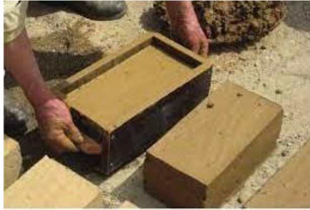
Figure 1-4 Production of adobe bricks [100]
