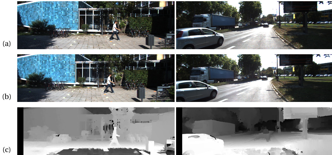
Figure 2.4 – Examples of DP modality with : a) RGB image from left camera ; b) RGB image from right camera ; c) Depth map from the stereo images, extracted with SGBM algorithm.
