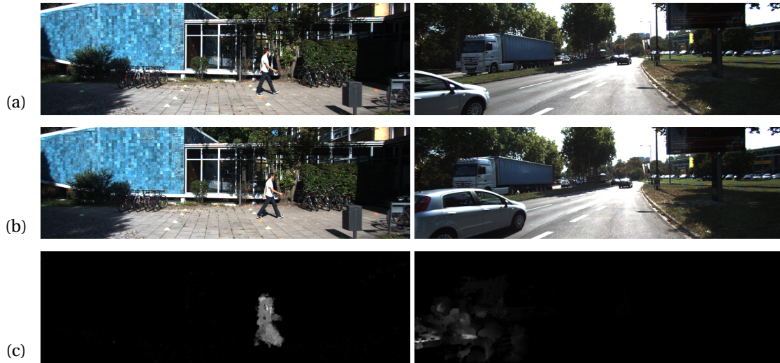
Figure 2.5 – Examples of OF modality with : a) RGB image from left camera ; b) RGB preceding image from left camera ; c) Optical flow map, from the 2 images, extracted with Farneback algorithm.
