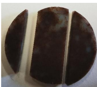
Figure III.15: PEEK-PTFE sample made with Cycle 1. The black-brown color indicated the degradation occurred in the process.
