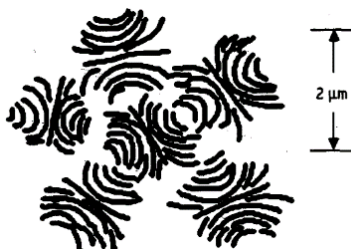
Figure II.24: Sheaflike structure of PEEK Spherulite according to Chu et al 123
