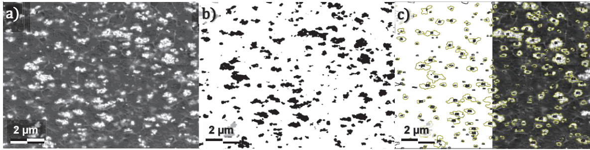
Figure 2.21: Example of Image analysis with a) the raw SEM image obtained in chemical contrast, b) the same image after binarization and c) the particle analysis partially overlaid on the raw images.
