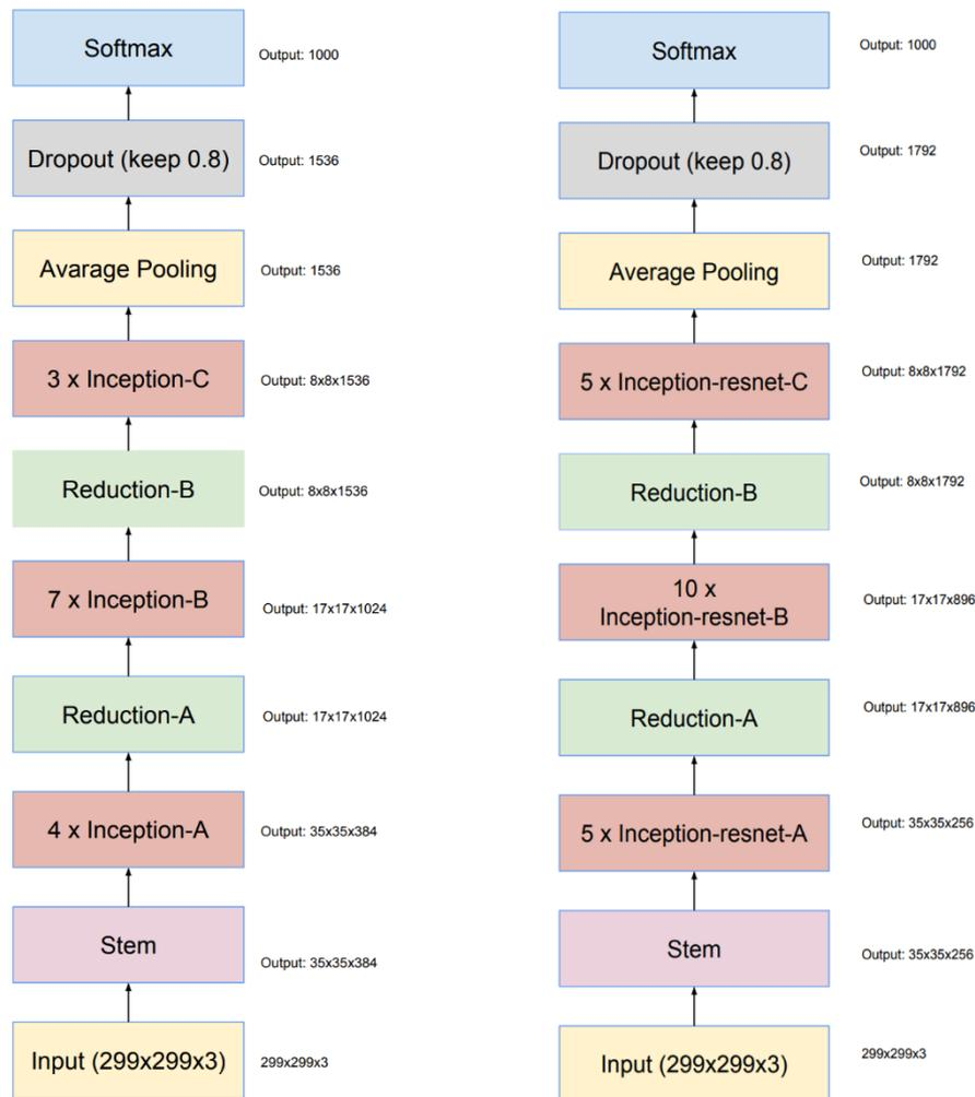
Figure 18: Entire inception-v4 (left), Inception-ResNet-v1 and Inception-ResNet-v2 (right) model architectures. The Inception-ResNet-v1 and Inception-ResNet-v2 models have the same architecture but their underlying modules differ. For more information on underlying modules (Inception(resnet)-A, Inception(resnet)-B, Inception(resnet)-C and Reductions) please refer to the original paper. (Figure from [SIVA16])
