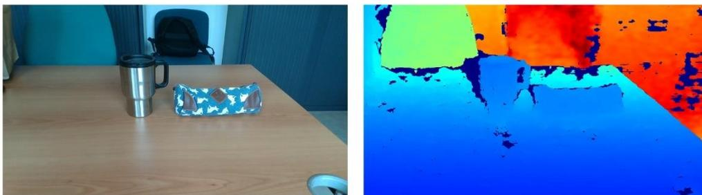
Figure 1: The RGB-D cameras provide a color (RGB) image alongside a depth map. The depth map indicates per pixel how far away objects are from the camera. This data is captured by Intel Realsense D435 camera. The depth map is colorized for better visualization.
