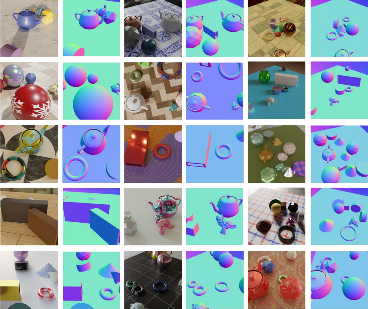
Figure 34: Dataset generated by our scene generator to be used for training the normal estimation network
