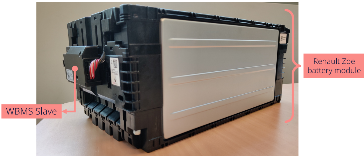
Figure 3.8 – Renault Zoe battery module connected to a TI WBMS slave which is inside the default Renault BMS slave box.
