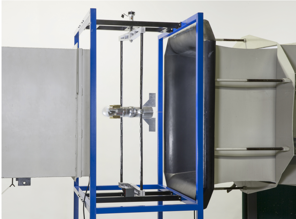
Figure 3.42 – Overview of the HIL projectile on its gimbal in wind tunnel [Strub, 2016]
