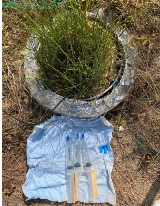
Figure II-6 Collection of pore water with syringes from 5, 15 and 30 cm depth of mesocosms.
