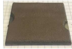
S-14Cr2W-YTi-0.2O-CS-N Brut de projection
