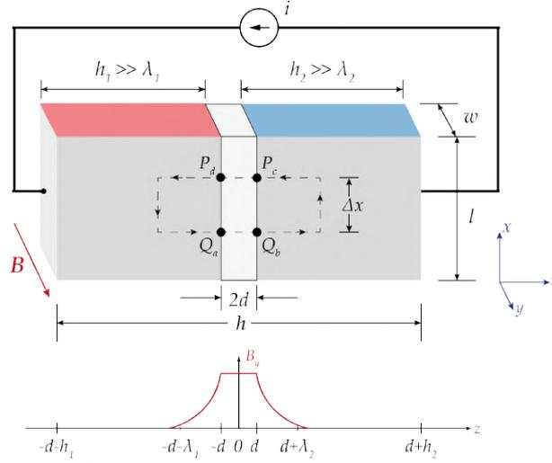
Figure 1.13: **Cross section of a Josephson junction.** The current flows in the  $x$ -direction, the magnetic field is applied in  $y$ -direction. The dashed line indicates the closed contour of integration. At the bottom, the decay of the magnetic field in the junction electrodes over the penetration depth is illustrated.
