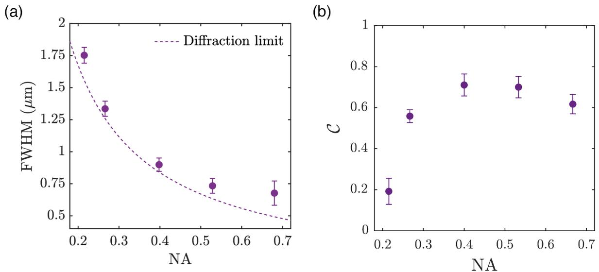
Figure 3.12:  $NA$  dependent FWHM and Contrast. Error bars translates variations from one vortex to another. (a) Vortex FWHM as a function of the effective  $NA$ . The diffraction limited FWHM is given by the dashed curve. (b) Vortex contrast  $\mathcal{C}$  as a function of the effective  $NA$ . There is a optimal  $NA$  that provides both a reasonable FWHM and contrast.
