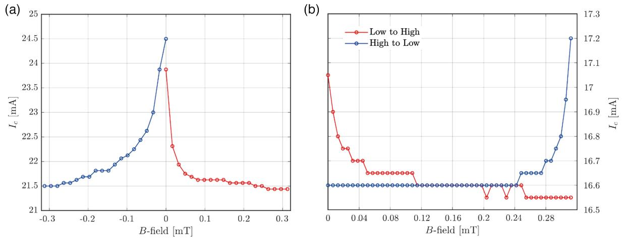
Figure 4.5: **SQUID magnetic field dependence.** (a) Magnetic field sweep from 0 to 0.3 mT and 0 to -0.3 mT, reversing the current direction in the coils. (b) Forward (low to high) and backward (high to low) sweep of the magnetic field. The measurements are performed at 7K and show decaying  $I_c$  at the beginning of the measurement with small change in the critical current.
