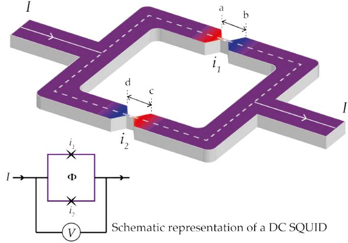
Figure 1.15: **SQUID.** Two Josephson junctions connected in parallel by a superconducting loop. The supercurrents across junctions  $a \rightarrow b$  and  $c \rightarrow d$  are labelled ( $i_{1/2}$ ). The enclosed flux threading the loop is given by  $\Phi$ . The path of integration  $C$  is shown by the dashed line.
