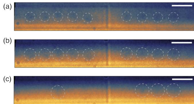
Figure 4.18: **Vortex depinning near junction.** Vortices near the junction remain pinned above the  $I_c$  determined from the transport measurement. Here MO images of the vortices (dark spots) are taken corresponding to the condition of  $I_{app} =$  (a) 3 mA, (b) 6 mA, and (c) 10 mA are applied. Vortices become unpinned at about 10 mA, 4 times larger than the  $I_c$ . Scale bars are 5  $\mu\text{m}$ .
