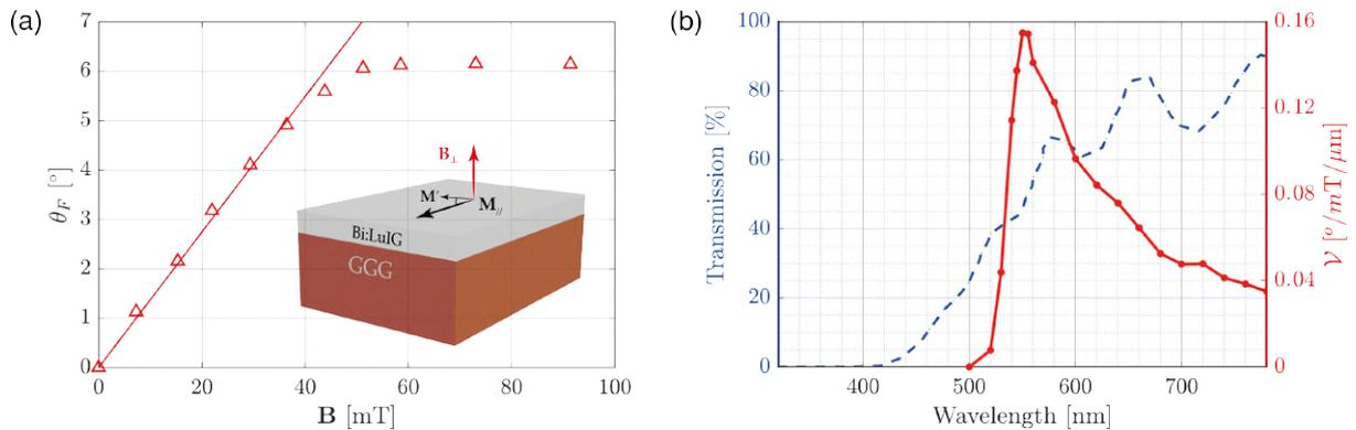
Figure 2.4: **Bi:LuIG magneto-optical characterisation.** (a) Faraday rotation for a  $2.5 \mu\text{m}$  Bi:LuIG MO indicator at 532 nm. The magnetisation ( $\mathbf{M}_{\parallel}$ ), applied magnetic field ( $\mathbf{B}_{\perp}$ ) and the local disordered magnetisation ( $\mathbf{M}'$ ) vectors are illustrated in the inset. (b) The wavelength dependence of the Verdet constant and transmission are plotted to illustrate an optimal measurement wavelength of 550 nm.
