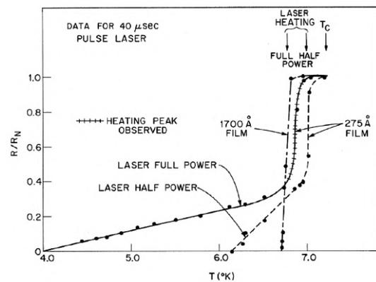
Figure 4.2: **Light induced Josephson characteristics.** Photo-induced changes in the resistive state of a Pb film [12]. The high temperature coefficient of resistance of Pb makes changes due to optical heating easy to detect.
