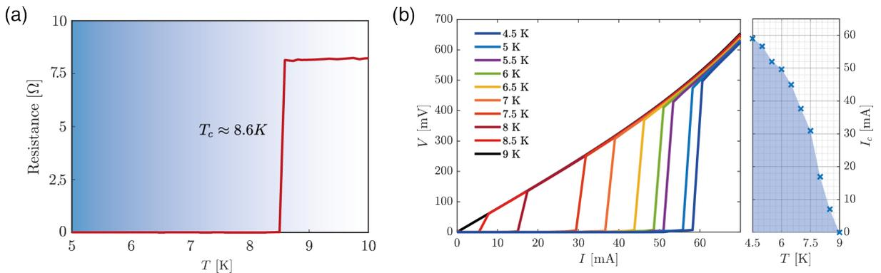
Figure 4.4: **SQUID critical transitions**(a) Resistive transition of device with a  $T_c \sim 8.6$  K and  $R_N \sim 8 \Omega$ . (b) Current transition plotted as a function of temperature.  $I_c \sim 60$  mA at 4.5 K.
