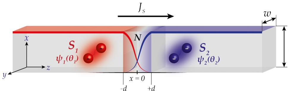
Figure 1.12: **Josephson junction.** (a) Schematic illustration of a conventional Josephson tunnel junction structure with two superconducting electrodes ( $S_{1/2}$ ) coupled by a tunneling barrier. The supercurrent density ( $J_S$ ) traverses the junction from  $S_1$  to  $S_2$ . The coupling of the superconducting wave functions  $\psi_{1/2}(\theta_{1/2})$  is shown as decay and overlap in the barrier region.
