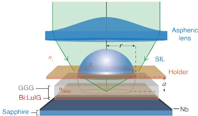
Figure 3.3: **Effective sSIL.** A hemisphere lens imposed on the MO indicator creates an effective sSIL geometry. A holder is used to maintain the SIL and indicator.
