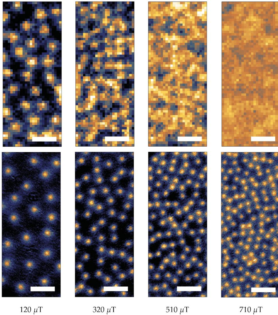
Figure 3.9: **B-field dependent single vortex imaging.** Vortices imaged in a magnetic field of  $B_{app} = 120$  to  $710 \mu\text{T}$  without (top) and with (bottom) the SIL. With the increased resolution previously unresolvable vortices are distinctly isolated. The scale bars are  $5 \mu\text{m}$ .
