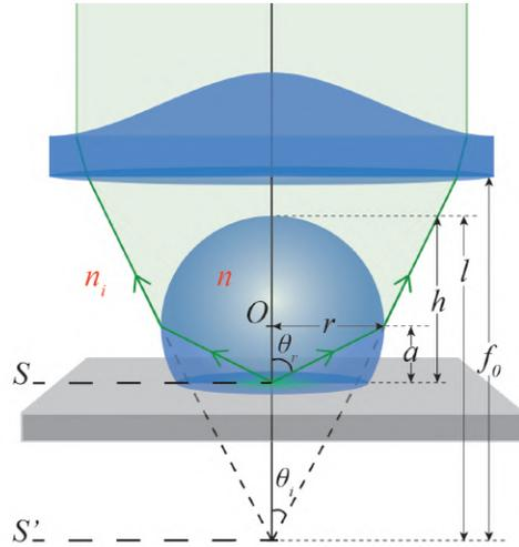
Figure 3.2: **super-Hemisphere SIL (sSIL)**. A super-Hemisphere requires an additional thickness  $a$  for a total SIL height  $h$ . The object  $S$  and virtual image  $S'$  planes appear at the bottom of the SIL and a distance  $l$  from the top of the SIL, respectively.
