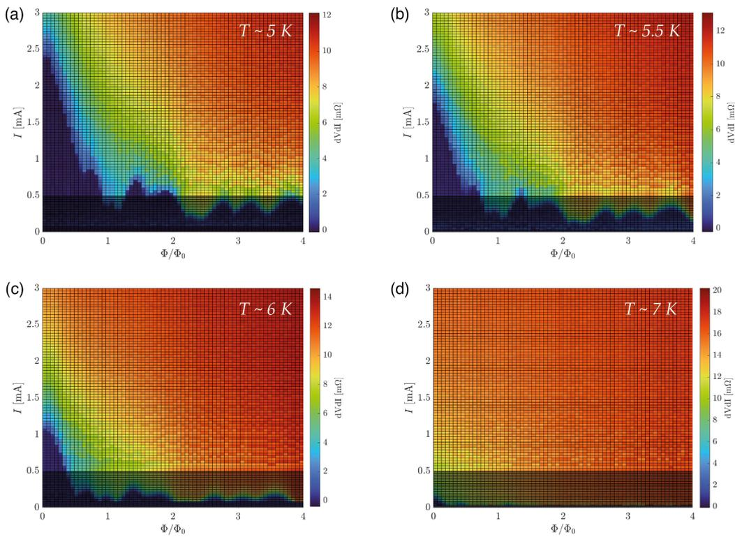
Figure 4.16: **Magnetic field dependence with temperature.** Fraunhofer oscillation patterns measured at temperatures  $T \sim 5, 5.5, 6$  and  $7$  K in (a-d), respectively. The measurements are performed with no vortices present within the optical FOV ( $\sim 60 \mu\text{m}$ ). The distortions in the pattern persist and the amplitude of the oscillations diminish with increasing temperature.
