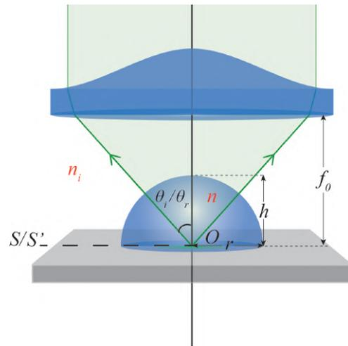
Figure 3.1: **Hemisphere SIL (hSIL)**. Hemispherical solid immersion lens with a radius  $r$  and height  $h$ . The object  $S$  and image  $S'$  plane coincide at the bottom of the lens on the optical axis at point  $O$ .
