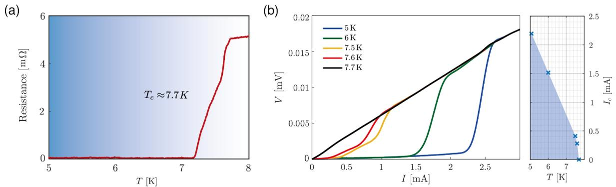
Figure 4.14: **Critical transitions**(a) Resistive transition of device with a  $T_c \sim 7.7\text{K}$  and  $R_N \sim 5\text{m}\Omega$ . (b) Current transition plotted as a function of temperature.  $I_c \sim 2.3 \text{ mA}$  at  $5\text{K}$ .
