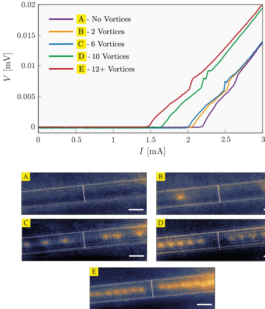
Figure 4.17: **Vortex imaging and IV measurement.** Vortex image correlated IV curves are obtained. Image (A) is cooled with a compensating field to remove the Earth's field. In images (B-E), vortices are trapped within the devices with field cooled conditions of 0.52, 0.63, 0.73 and 0.84 mT. Corresponding IV curves show changes in the  $I_c$  and difference in the shape of the transition related to the vortex distribution. The scale bars are 5  $\mu\text{m}$ .
