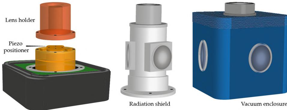
Figure 2.2: **Optical cryostation.** The outer components of the optical cryostation is illustrated. The sample platform is mounted on a piezo positioned with thermal link cables connected to the brass cylinder thermalised to the second stage ( $\sim 3K$ ). The lens is held by a copper holder mounted on the brass cylinder. The radiation shield is then fixed, followed by the vacuum enclosure. Optical access is enabled through glass windows on the top and all four sides.
