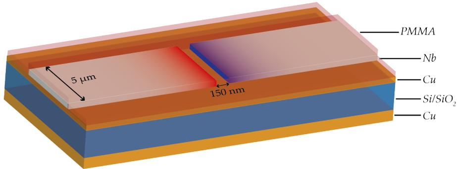
Figure 4.13: **Variable thickness bridge - SNS junction.** The junction length is  $5 \mu\text{m}$ , with a width of  $150 \text{ nm}$ . A layer of  $200 \text{ nm}$  PMMA is deposited on top to protect the Cu from oxidation. Each of the electrodes branches into a pair of contact pads, and the transport properties are measured by applying a current and measuring the voltage drop across the junction in a 4-point configuration.
