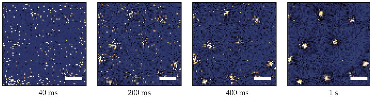
Figure 3.7: **Integration time of single-shot images.** Single-shot images taken at 40 ms, 200 ms, 400 ms and 1 s. Individual vortices can be resolved at a sub-second scale with good SNR. The scale bars are  $2 \mu\text{m}$ .
