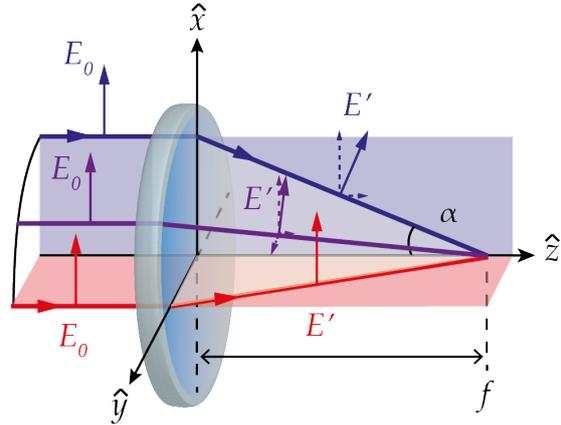
Figure 3.11: **Polarisation in high-NA system.** Focusing linearly polarised light by a high-NA lens introduces off-axis projections in the polarisation profile. For MOI, polarisation quality is critical to obtaining image contrast.
