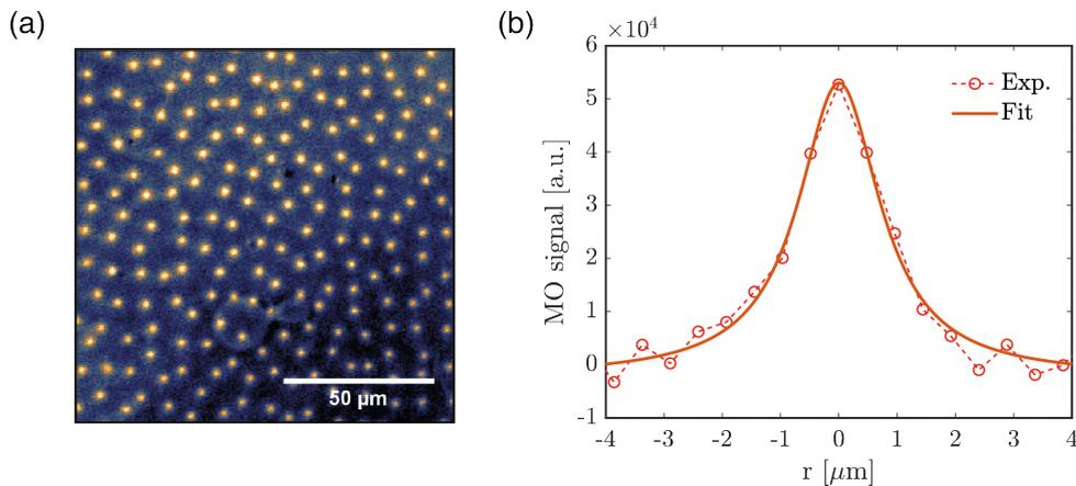
Figure 2.6: **Vortex imaging.** (a) An image of single vortices resolved using the MOI set-up in a Nb film of 100 nm, taken at 4.5K in a field of  $\sim 30 \mu\text{T}$ . (b) Intensity profile of a single vortex with a FWHM size of  $\sim 1.7 \mu\text{m}$ .
