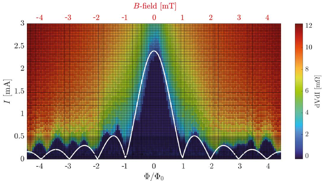
Figure 4.15: **Magnetic field dependence.** The magnetic field is swept from -3 to 3 mT, acquiring a full IV curve at each increment. Fine increments are taken at low current values. The colour scale shows the  $dV/dI$  intensity. The white curve is the interference for an ideal junction of the calculated periodicity. Data acquired at  $T \sim 5\text{K}$ .
