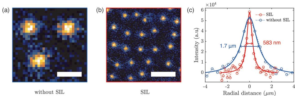
Figure 3.8: **FWHM.** (a) Single vortex imaging using the classic MOI method. (b) Single vortex imaging using the SIL integrated MOI method. (c) Lorentzian fit for the smallest imaged vortices for the two configurations. The vortices are resolved with a FWHM of  $1.7 \mu\text{m}$  and  $583$  nm without and with the SIL, respectively. The scale bars are  $5 \mu\text{m}$ .
