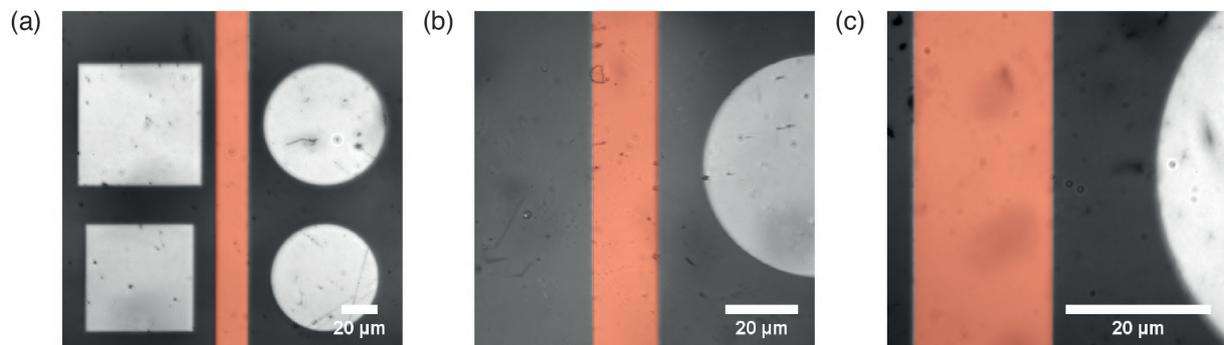
Figure 3.5: **SIL magnification.** Images taken of features on a device. All images show an area of  $450 \times 450$  pixels, with the shaded orange feature having a physical width of  $20 \mu\text{m}$ . (a) Without the SIL and GGG, (b) in the hSIL geometry and (c) with the GGG in the sSIL geometry.
