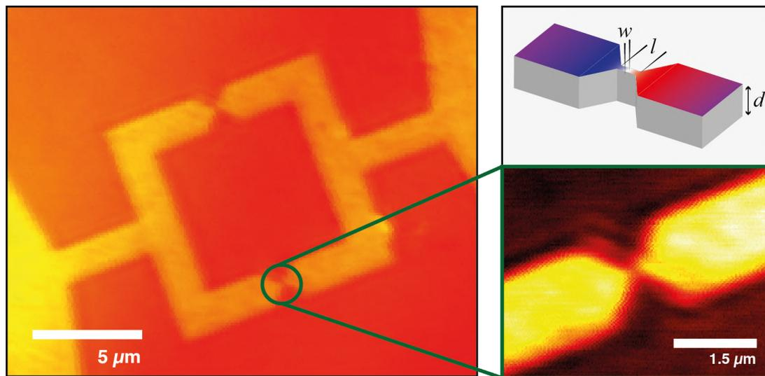
Figure 4.6: **SQUID confocal image.** A scanning confocal image of the device area is mapped using the SIL. The weak-link region can be further isolated and using finer steps, a high resolution image of the structure can be mapped. The region of the bridge cannot entirely be resolved as the dimensions fall below the resolution capability of the system.
