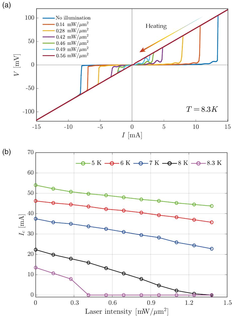
Figure 4.7: **SQUID IV modulation.**(a) Optically induced modulation of the  $I_c$  of one weak-link at  $T \sim 8.3\text{K}$ . Within a range of impinging illumination intensities the  $I_c$  of the device can be suppressed completely and recovered by cutting the illumination. (b) Suppression of the device  $I_c$  at  $T = 5\text{-}8.3\text{K}$ . The suppression is limited at low temperatures even with strong illumination.
