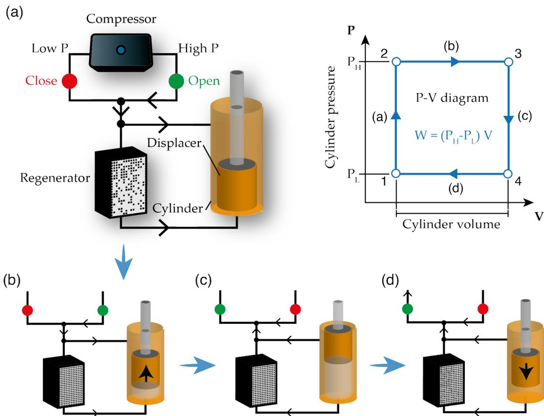
Figure 2.1: **Gifford-McMahon refrigeration scheme.** The four stages of the GM cooling cycle. The inset illustrates a Pressure-Volume plot that follows the thermodynamic cycle. The useful cooling power  $W$  is the product of change in pressure ( $P_H - P_L$ ) and volume  $V$ .
