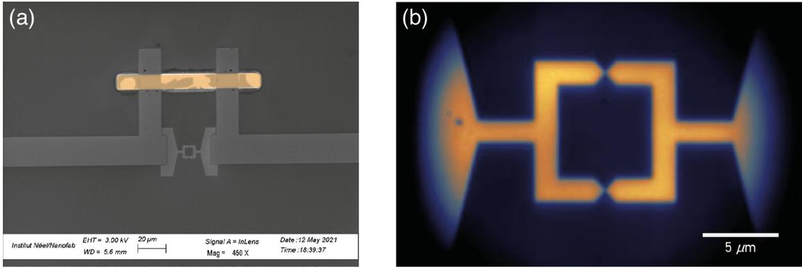
Figure 4.3: **Dayem bridge SQUID.** (a) SEM image and (b) Wide-field optical image of the SQUID. The bridge dimensions in the samples varied from  $l \sim 100 - 200$  nm and  $w \sim 50 - 70$  nm. The inside of the SQUID loop is  $6 \times 6 \mu\text{m}^2$  with  $1.5 \mu\text{m}$  wide electrodes. The device has been shunted with a gold line, highlighted in the SEM image, to protect the device from accidental electrostatic damage.
