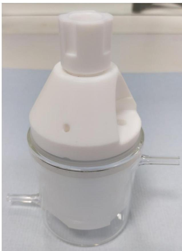
Figure II.7. Electrochemical cell designed with Kel-F and PTFE top.
