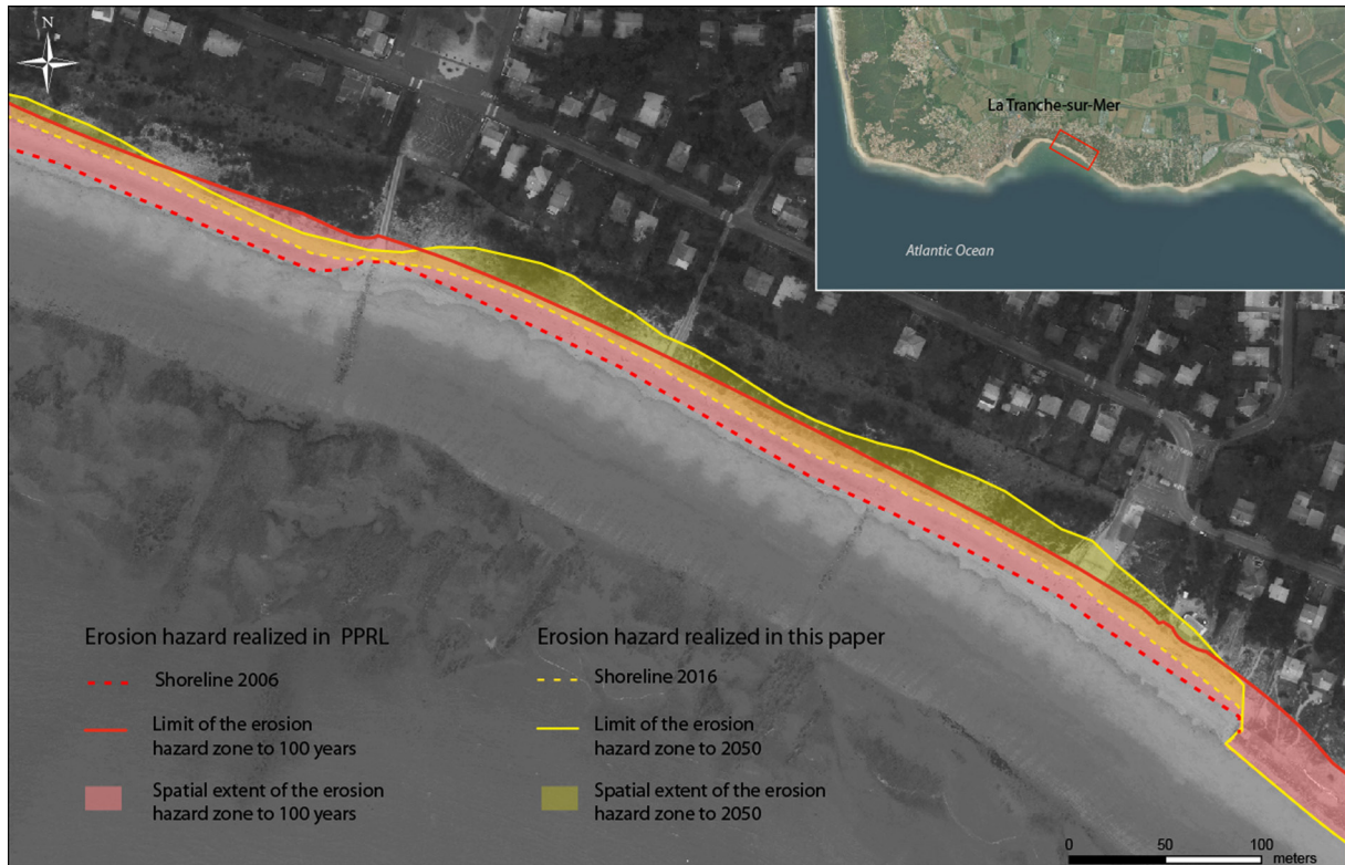
Figure 13 : Comparison of erosion hazard zones by 2050 and 2120. Clémenceau beach, La Tranche-sur-Mer.
