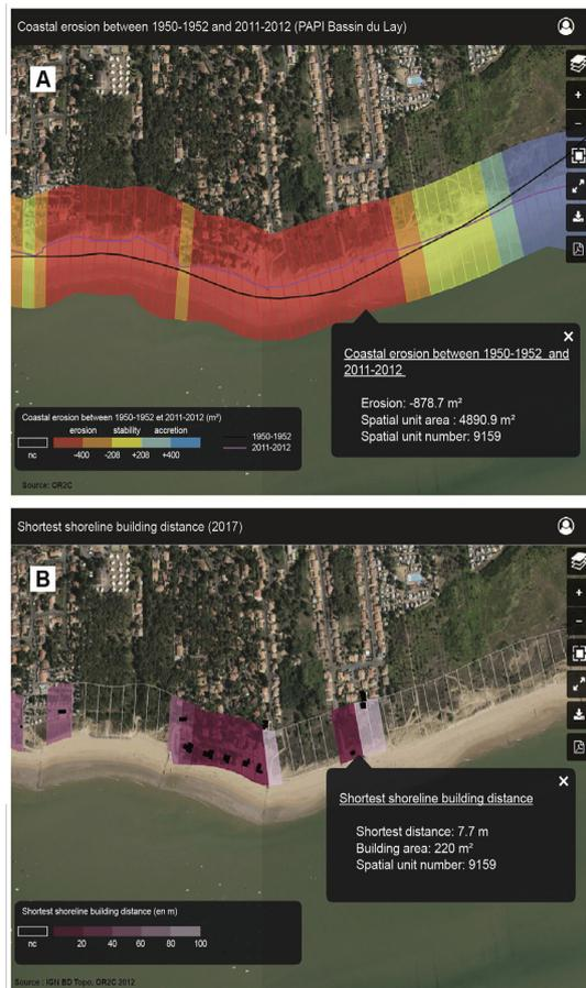
Fig. 7. Spatial display of two indicators from the MAP-RISC web-page located in the eastern coast of La Tranche-sur-Mer (Vendée). Per spatial unit: A. Coastal erosion (m<sup>2</sup>) with full spatial units; B. Shortest shoreline-building distance (m) with onshore spatial units.
