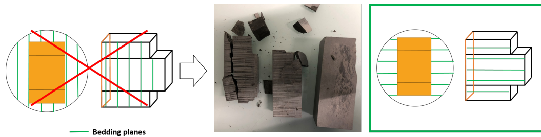
Fig. 5.7.: Green lines represent the bedding planes in the cross section of a core and in the sample. Schematic representation of the proper orientation of the interfaces with respect to the bedding planes naturally present in the rock.
