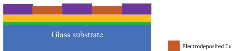
Fig. IV. 12. The representation of the wafer after Cu electrodeposition
