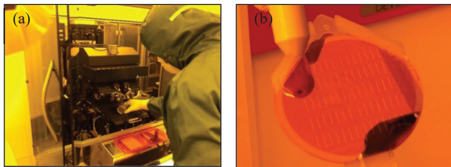
Fig. IV. 9. UV photolithography equipment (a): wafer mask alignment to the light exposure) and (b): the wafer after photoresist cleaning up
