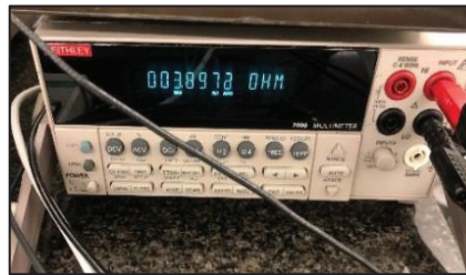
Fig. IV. 22. Digital multimeter (KEITHLEY 2100, 1kV3A, 6.5 digits) used for Resistance measurement
