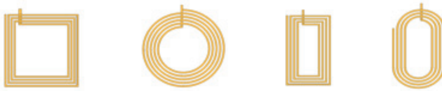
Fig. II. 4. The four geometries of micro-coil designed in CST MWS
