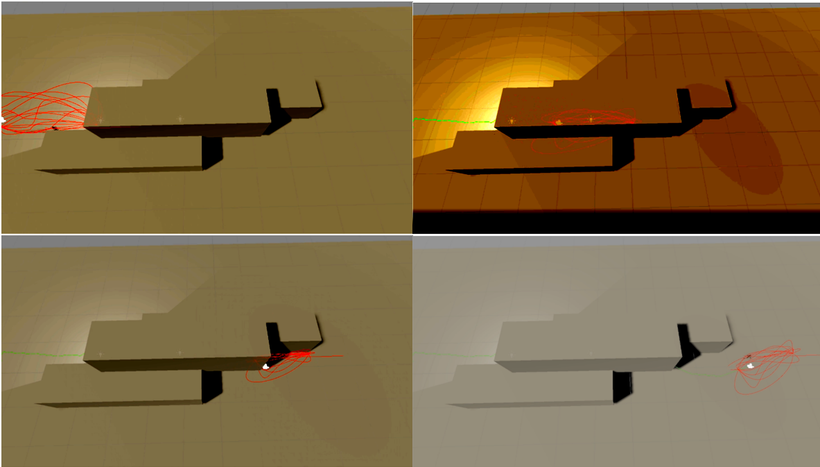
Figure 4.20 – Results on a scene with a corridor: we move the target through the corridor to illustrate how the animation space adapts to the environment. In red, we see 20 randomly picked trajectories from the animation space. In the first image ( i.e. upper left) there is wall only on the right of the character, and we can already see that the right of the animation space has shrunk. In the second image ( i.e. upper right), the character is surrounded by walls, and we can see that the animation space has shrunk in all directions. Finally, in the last two images as the character gets out of the corridor, the animation space widens to its original scales.
