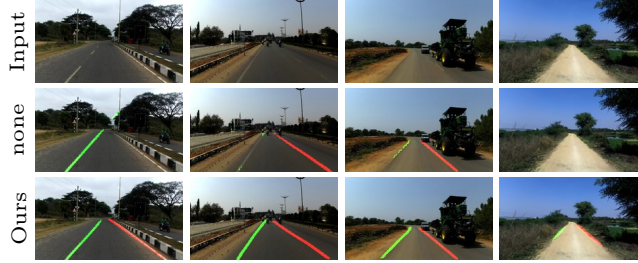
Figure 4.7: SCNN (Pan et al., 2017) lane detection on IDD (Varma et al., 2019). Training on generated images with degraded lanes makes existing lane detectors – such as SCNN (Pan et al., 2017) – resistant to scenes with damaged (first three columns) or no (last column) lane markings.
