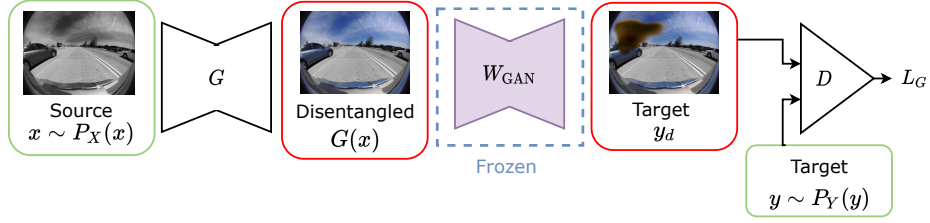
Figure 7.4: Neural-guided disentanglement. We exploit here a separate frozen GAN ( W_{GAN} ) which renders specific target traits (here, dirt) on generator G output images before forwarding them to the discriminator D . We do not show gradient propagation for simplicity.
