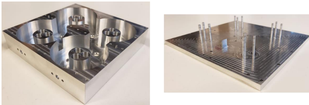
Figure IV.40 Fabricated filter k=3 . Body (left) and cover (right) parts
