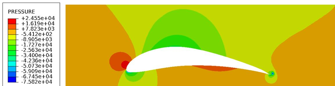
**(a)** Pressure isovalues around the Eppler 420 hydrofoil obtained with the fluid FSI model
