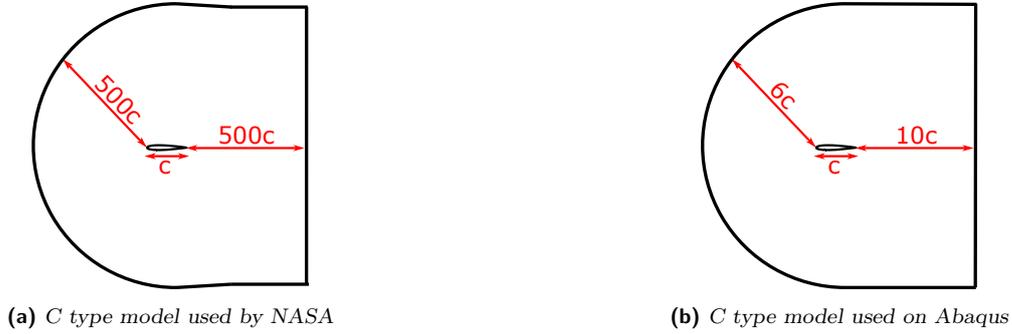
**Figure A.20.** *C-type models for airfoils*
