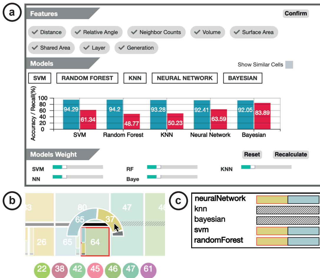
Figure 6.1 - The visualization design for our multiple machine learning models. (a) The overview of the model performance. Users can customize the features to train models. Also, they can change the model weights via the panel. (b) The detailed prediction of a specific cell (cell 64 as an example in this figure). (c) The model results of the target cell (cell 64) and the interested proposed sister cell (cell 37) being sisters.
