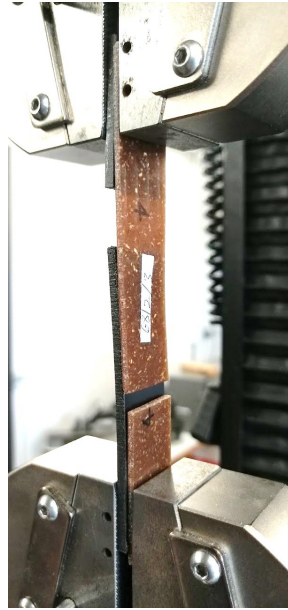
Figure 4.16: Lap shear test performed on Instron 1185 UTM.
