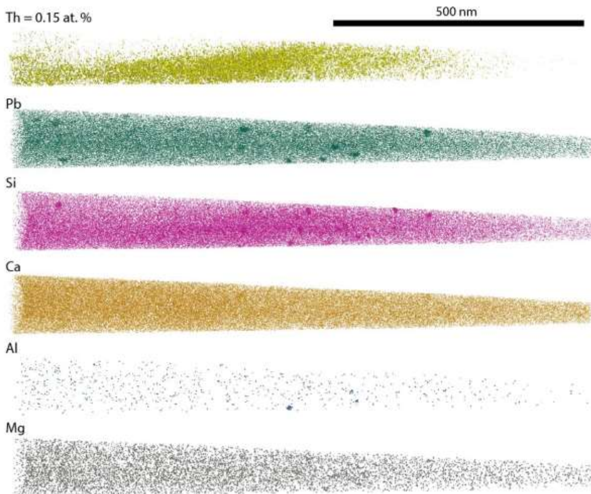
Figure VII-10: APT reconstruction of M16 specimen (location supplementary data 2 Fig. S4) targeting a thin Th-rich planar feature. Thorium isoconcentration at 0.15 at.% highlight the Th-rich network. Distribution of Pb and Si show a heterogeneous distribution forming clumps localized in the Th-rich network. Si enriches in the Th-rich network. Ca shows a slightly heterogeneous distribution forming clumps spatially correlated with some of the Pb-Si clumps and Al is heterogeneously distributed, highlighting Al enrichments in the Pb-Si clumps. One dot = one atom.
