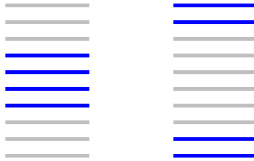
Figure 4.1: Evaluation of the AUC-ROC and AP on two rankings. Blue ( resp. grey) lines represent positive ( resp. negative) samples. While AUC-ROC behaves similarly on both cases ( AUC-ROC = \frac{1}{2} ), the average precision is equal to 0.43 on the left and 0.68 on the right, illustrating that AP favors the ranking that put (at least some) positives at the very top of the list.
