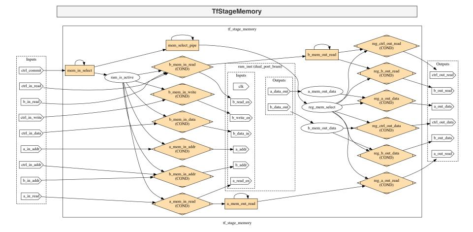
Figure C.6: Synchronization-oriented representation of *TfStageMemory* module
