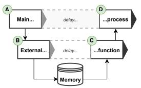
Figure 5.2: Example pipeline requiring delay for signal synchronization
