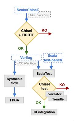
Figure 4.3: Chisel design and validation flow
