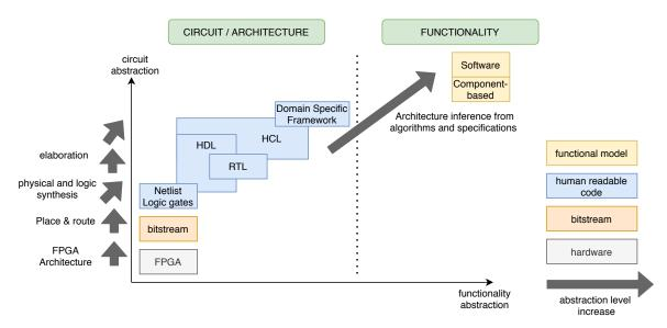
to instantiate base logic elements and to define their connections while the painful task of mapping the circuit to an FPGA architecture is left to a *place and route* tool.
