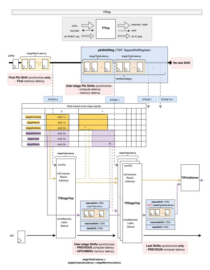
Figure C.1: Manual reverse engineering of Top-Level Tree Filters Hierarchy
