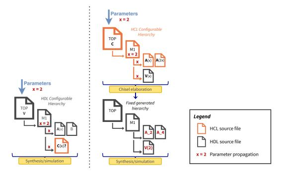
Figure 6.5: Parameter propagation compared in HDL and HCL hierarchies
