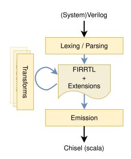
Figure 6.3: Main processing steps of sv2chisel
