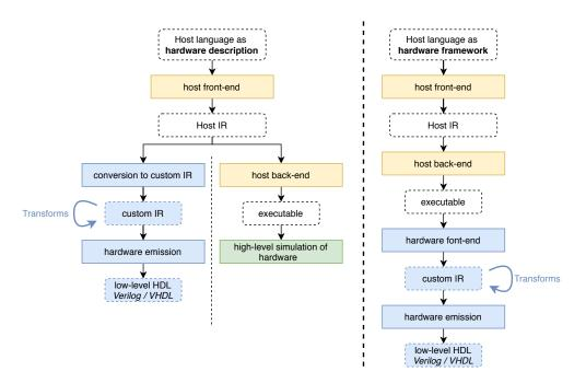
Figure 3.3: Implementation principles for embedded HCLs
