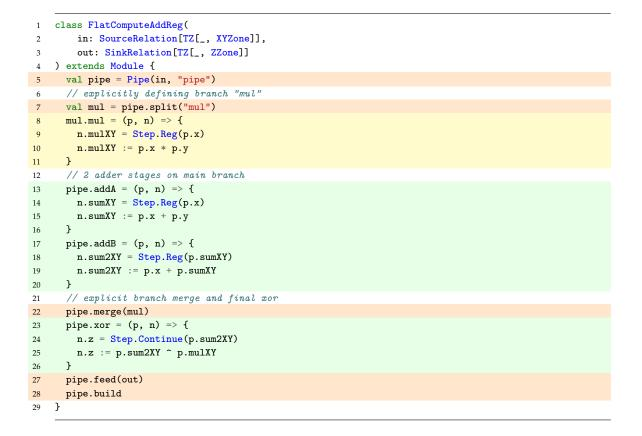
Figure 5.4: Running example implemented with our pipeline-oriented framework based on Chisel HCL
