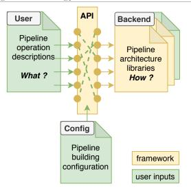
Figure 5.3: Decoupled pipeline description methodology
