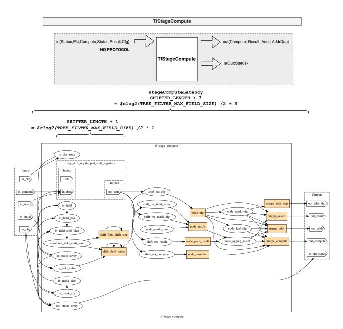
Figure C.3: Synchronization-oriented representation of the core compute submodule *TfStage-Top* of *Tree Filters* Hierarchy
