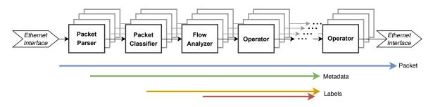
Figure 7.1: Coarse-grained generic architecture of network devices
