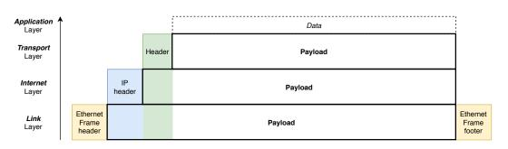
Figure 2.2: Typical IP packet structure in the *Internet protocol suite* (*TCP/IP*) model from *Link* layer to *Application* layer
