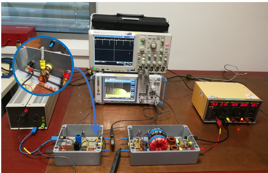
Figure II.56: Experimental validation of the Black Box model."Minus to ground" case. Minus to ground connection on the converter side can be seen in zoom.
