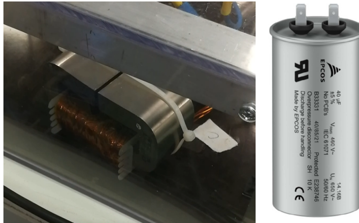
Figure I.28: View of inductors and capacitors used in experiments.
