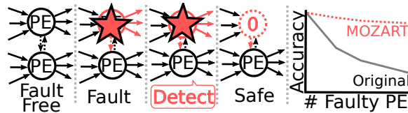
Figure 4.1: MOZART+ Provides On-Line Testing and Fault Masking with Graceful Degradation in Accuracy
