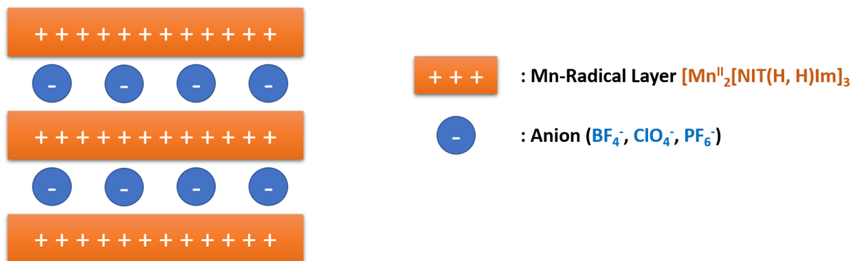
Figure 3.10: Schematization of how 2D manganese-radical layers and the anions are stacked in compounds similar to YI_OTf03. Manganese-radicals form 2D layers which are separated by the anions, whose size influences the interlayer separation distance. The chemical content of the layer is the same for all compounds, but different anions are inserted among them.
