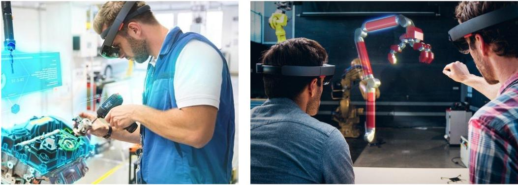
Fig. 1.1 The left picture gives an illustration of an AR operator being assisted by the AR assistance system while performing an assembly task. The right picture shows an illustration of operator teaching using an AR system. AR projects the learner into a context closer to reality than traditional learning methods. It makes the task easier for the assembler by more pleasantly displaying the instructions to be followed.
