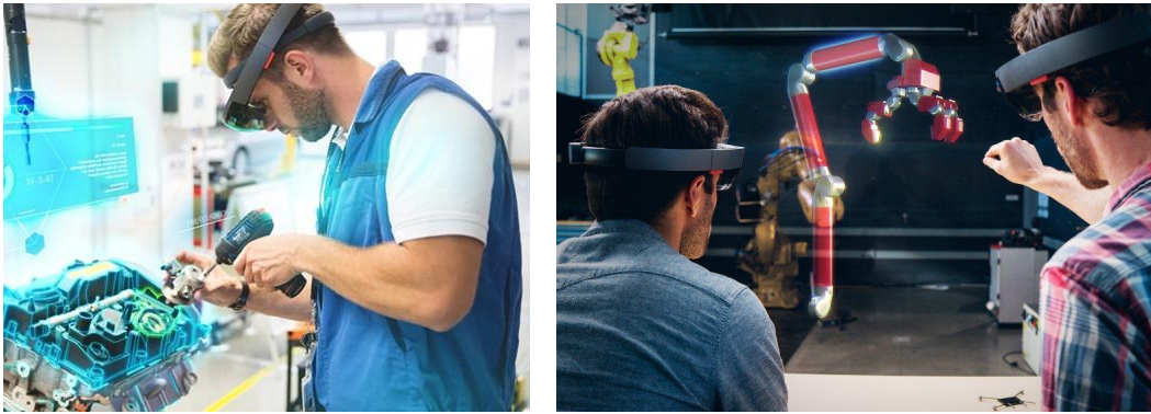
Fig. 1.1 The left picture gives an illustration of an AR operator being assisted by the AR assistance system while performing an assembly task. The right picture shows an illustration of operator teaching using an AR system. AR projects the learner into a context closer to reality than traditional learning methods. It makes the task easier for the assembler by more pleasantly displaying the instructions to be followed.
