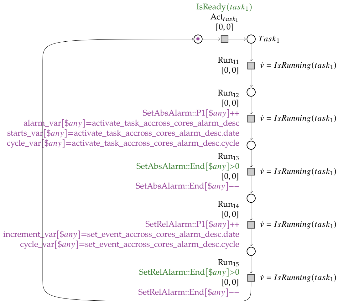
Figure 6.4: Task_1 model of the mc\_alarm\_s1 test sequence.
