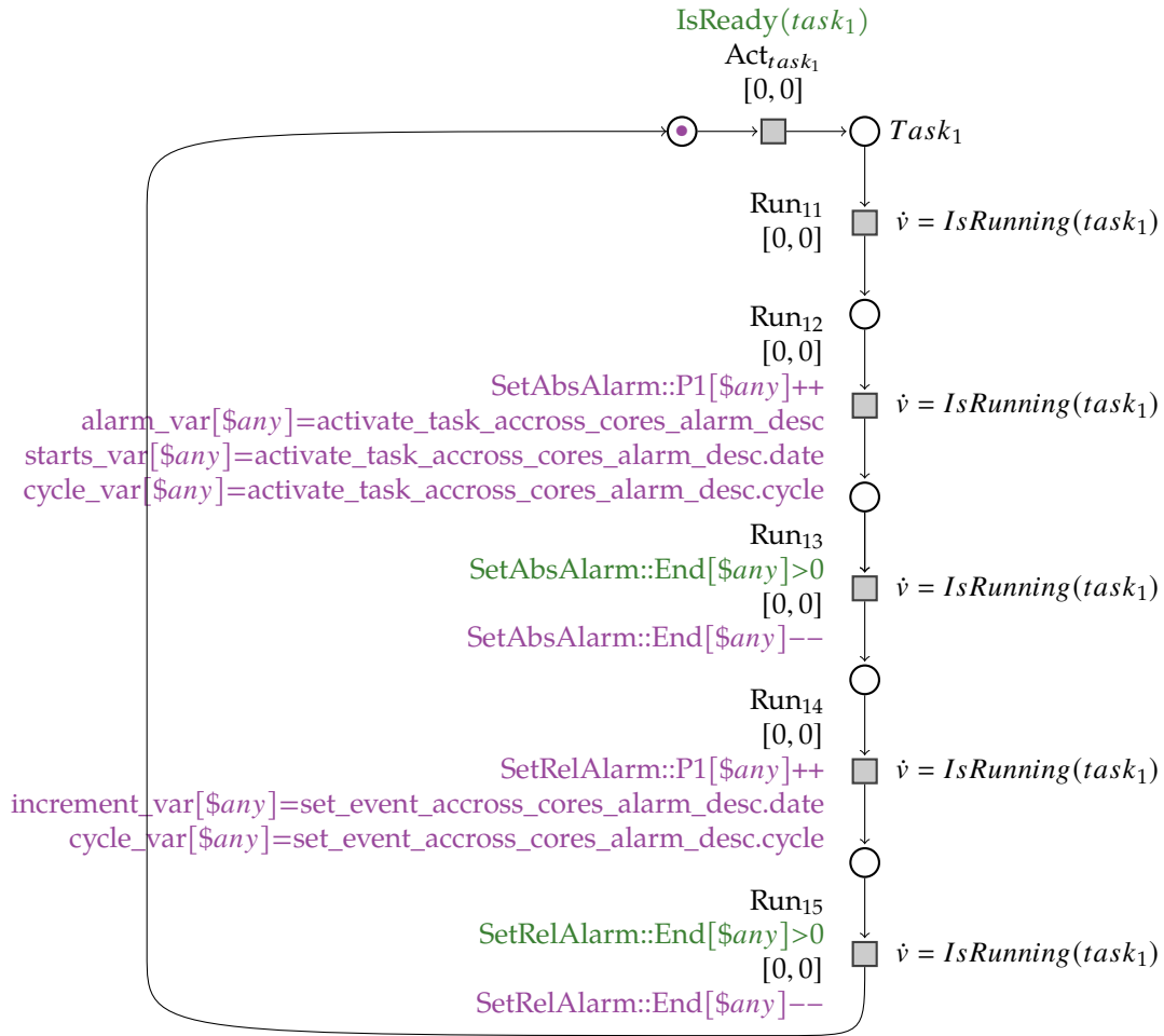
Figure 6.4: Task 1 model of the mc_alarm_s1 test sequence.
