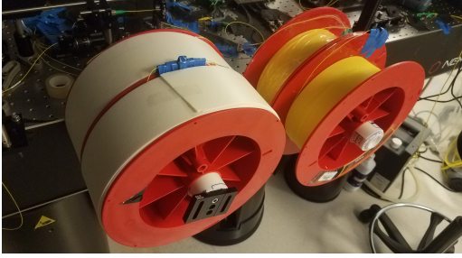
(a) With no insulation (right), and partial insulation (left).
