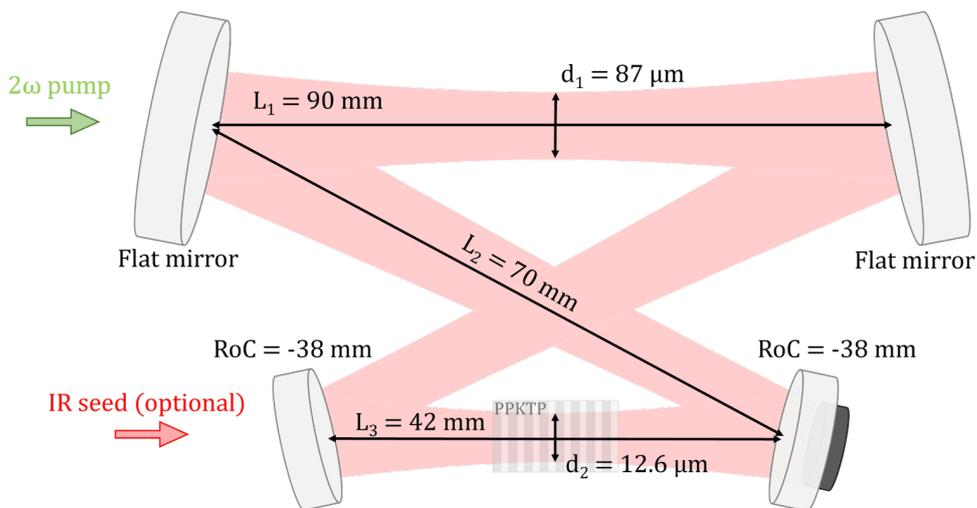
Fig. IV.16 Schematics of the OPO bow-tie cavity geometry
