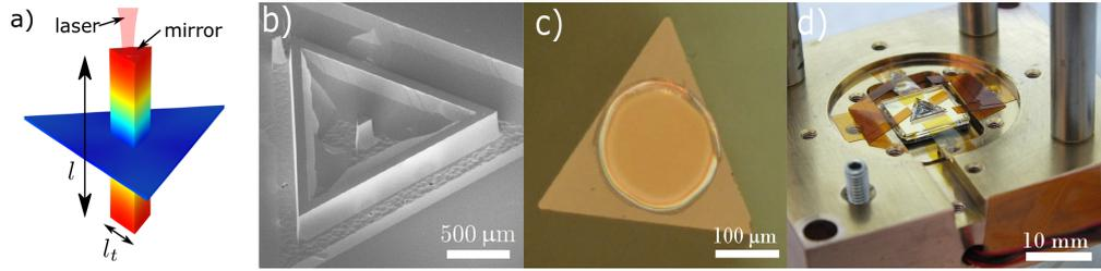
Fig. III.3 **The micro-pillar resonator.** a) Finite-element simulation of the fundamental elongation mode. Displacement is represented by the color scale. Mechanical stress is minimized at the mirror location. b) Scanning Electron Micrograph view of the pillar and its isolation frame. c) Optical view of the mirror coated on the top face of the resonator. d) View of the resonator glued on copper pieces coated with gold and ready to be mounted inside the cryostat.
