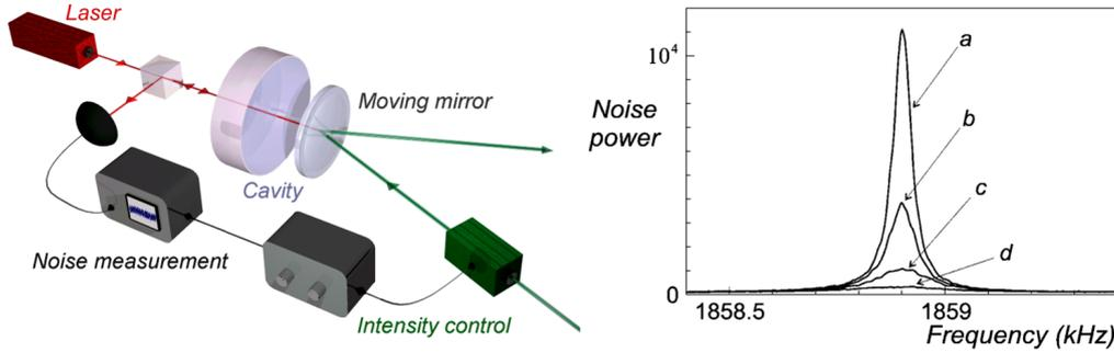
Fig. I.6 **First feedback cooling experiment performed at LKB.** Left: Experimental setup. The field reflected by the cavity is used to probe the mirror position. An auxiliary laser beam, reflected on the end mirror, is used to apply a feedback force on the mirror and counter the Brownian noise. Right: Thermal noise spectrum of the mirror without feedback (a) and with increasing feedback gains (b) to (d).
