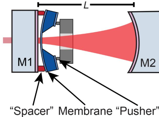
Fig. V.4 *The MATE cavity experiment from Jack Sankey’s group. It is made of an input mirror M1, 21- $\mu\text{m}$  thick spacers, a membrane, piezo-actuated pushers, and a “backstop” mirror (not to scale). The length  $L = 10$  cm between M1 and M2 is tuned with piezo actuators on M2. Figure from [24].*
