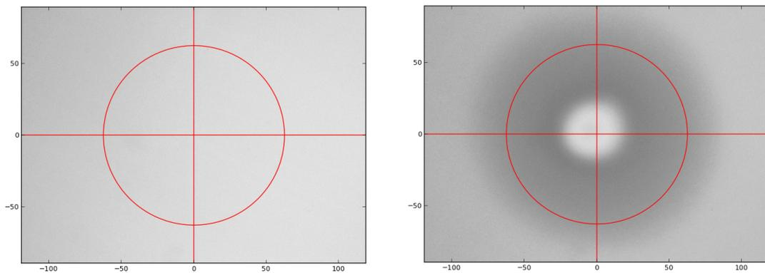
Fig. III.9 *Interferometric profile of a Suprasil sample before and after a  $\text{CO}_2$  laser shot of 90 ms. We have obtained a concave structure with a  $60\text{-}\mu\text{m}$  diameter and a radius of curvature of 1.3 mm.*
