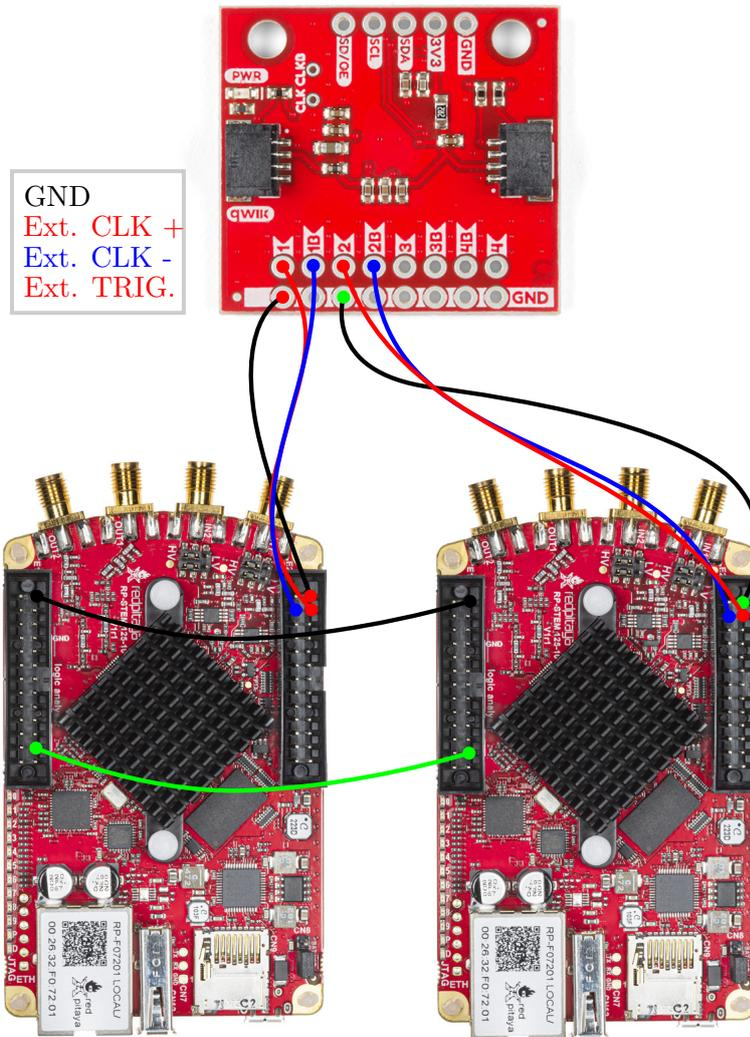
Fig. IV.28 **Two synced RedPitayas.** The small red board generates the external clock signal and the green cable between the two RPs ensure that the IQ modules keep a constant phase relationship.
