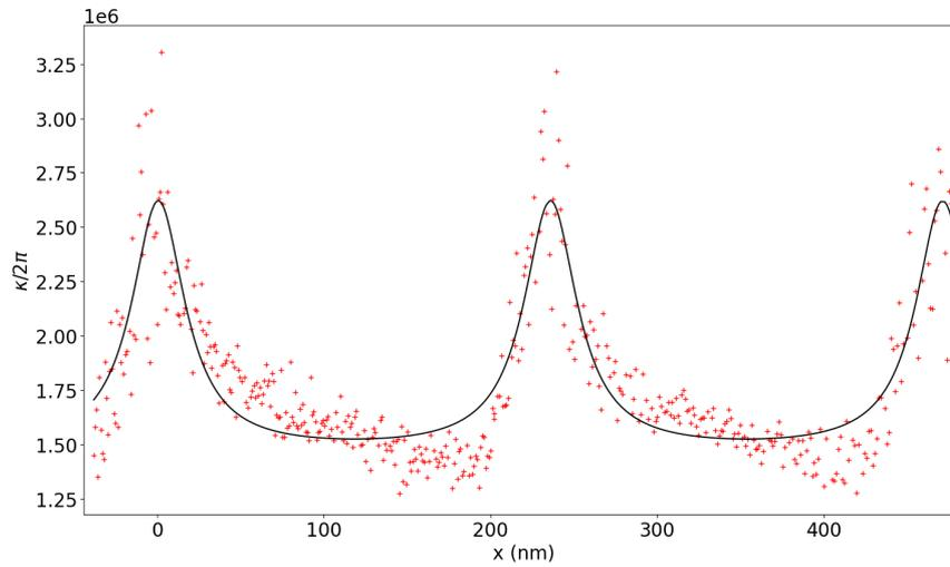
Fig. V.10 **Decay rate of MATE cavity as a function of the membrane position.** We see that as the membrane goes through the nodes and antinodes of the standing wave inside the cavity, we increase or decrease the decay rate of the cavity.
