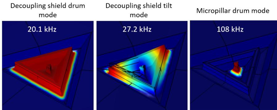
Fig. III.4 *Finite-element simulations of the parasitic low-frequency modes of the micro-pillar. For high optical power, vibrations at these frequencies drastically increase and make the cavity impossible to properly lock at resonance.*
