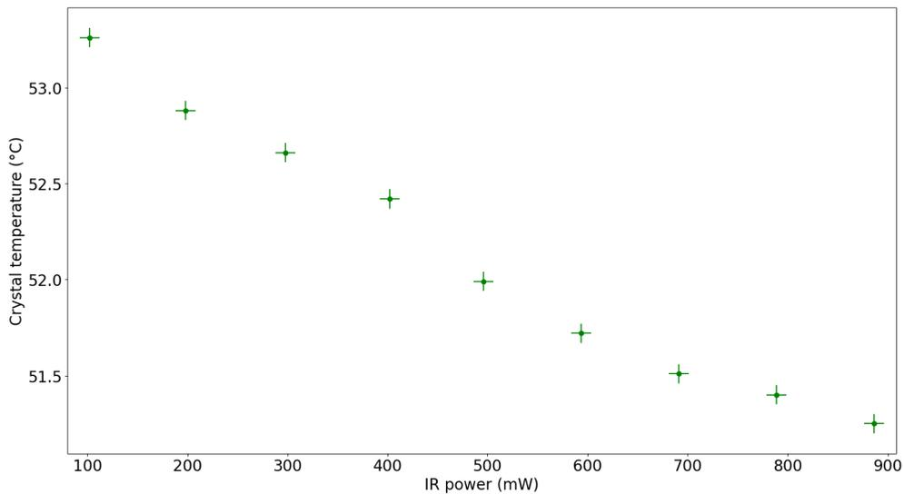
Fig. IV.13 **Optimal set-point temperature of the temperature controller for non-linear gain as a function of the IR pump power.** We can see that as we increase the amount of IR power inside the cavity, we heat up the crystal and we need to compensate with the temperature controller. We observed that those values tend to also depend on the temperature of the room.
