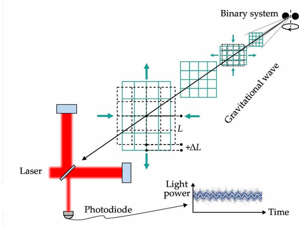
Fig. I.1 **Principle of interferometric GW detection.** A binary system (typically neutron star or black holes) creates a gravitational wave that will travel to earth where it will cause a variation of the optical path in the two arms creating an oscillation on the amplitude measured by the photodiode. Figure adapted from [12].
