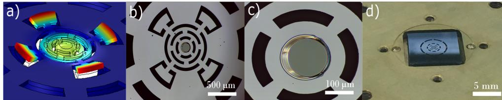
Fig. III.6 **The LKB wheel resonator.** a) Finite-element simulation of the mechanical mode of interest. Displacements are represented by the color scale. b) and c) Views of the resonator taken with an optical microscope for various magnifications. d) View of the resonator glued on copper pieces coated with gold and ready to be mounted inside the cryostat.
