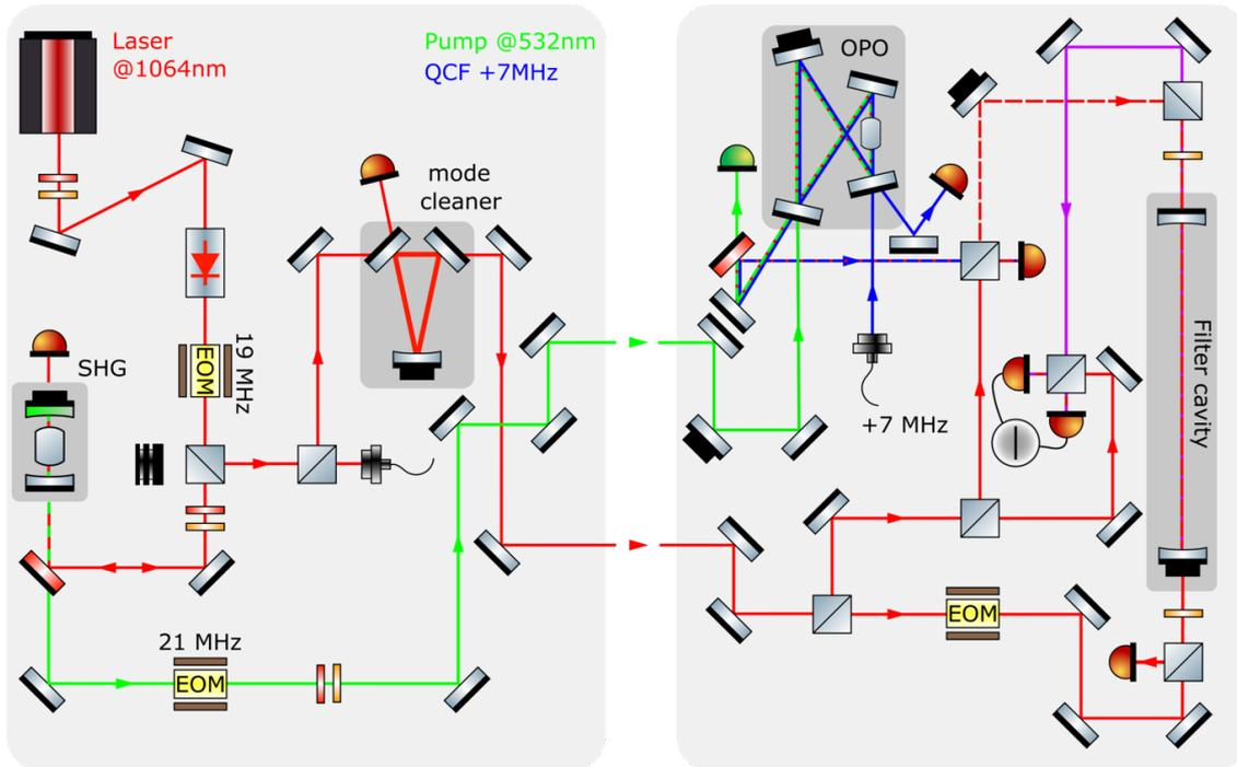
Fig. IV.22 *Simplified optical setup with all the principal elements.* EOM stands for *Electro-Optic Modulator*. Those are used to generate phase modulation for the PDH locks mentioned in section IV.7. The detuned coherent control field is represented in blue, the vacuum squeezed field is represented in dashed red and frequency dependent squeezing is represented in purple.
