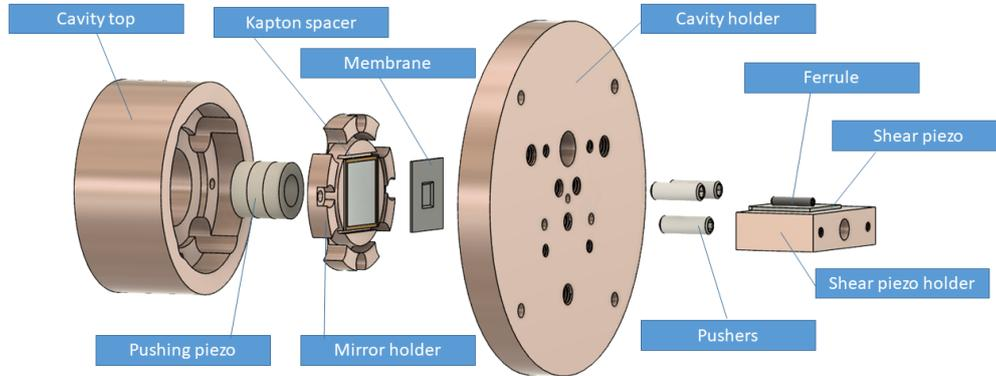
Fig. V.6 Exploded view of the fiber MATE cavity design. The "cavity top" and "mirror holder" parts are the same as before. The "cavity holder" has been modified with extra threads for the "pushers", a hole to fit the ferrule and 2 extra threads to put screws holding the "shear piezo holder". The shear piezo holder has a hole in the middle for the pusher.
