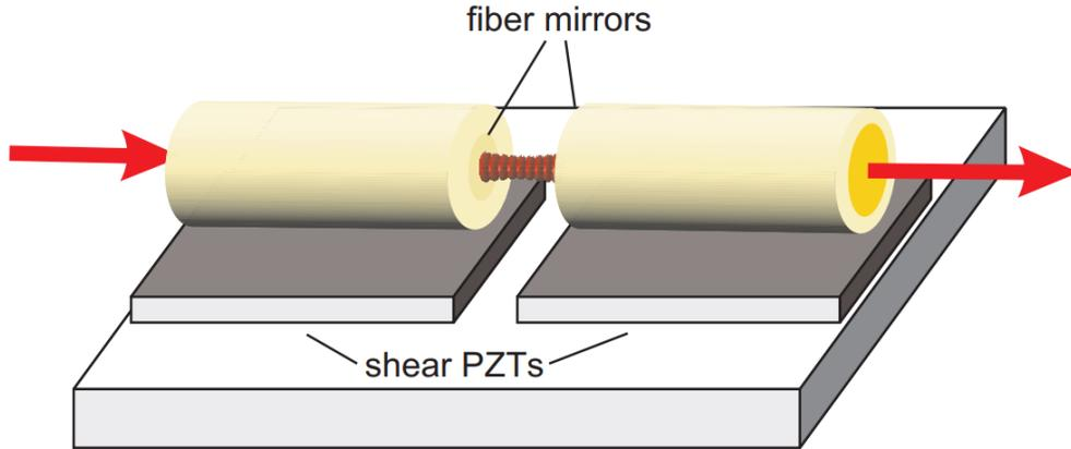
Fig. V.5 *Miniature mounts for a tunable Fiber Fabry-Perot Cavity by Jakob Reichel's group. Piezoelectric transducers are used to scan the cavity length. All other alignment is done during assembly. Figure from [76].*
