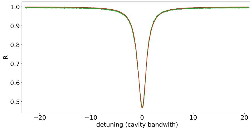
Fig. IV.5 Reflection signal of the MCIR cavity obtained upon scanning the length of the cavity using the piezoelectric transducer glued to one mirror. We can extract  $R_0$  using a Lorentzian fit of the data.
