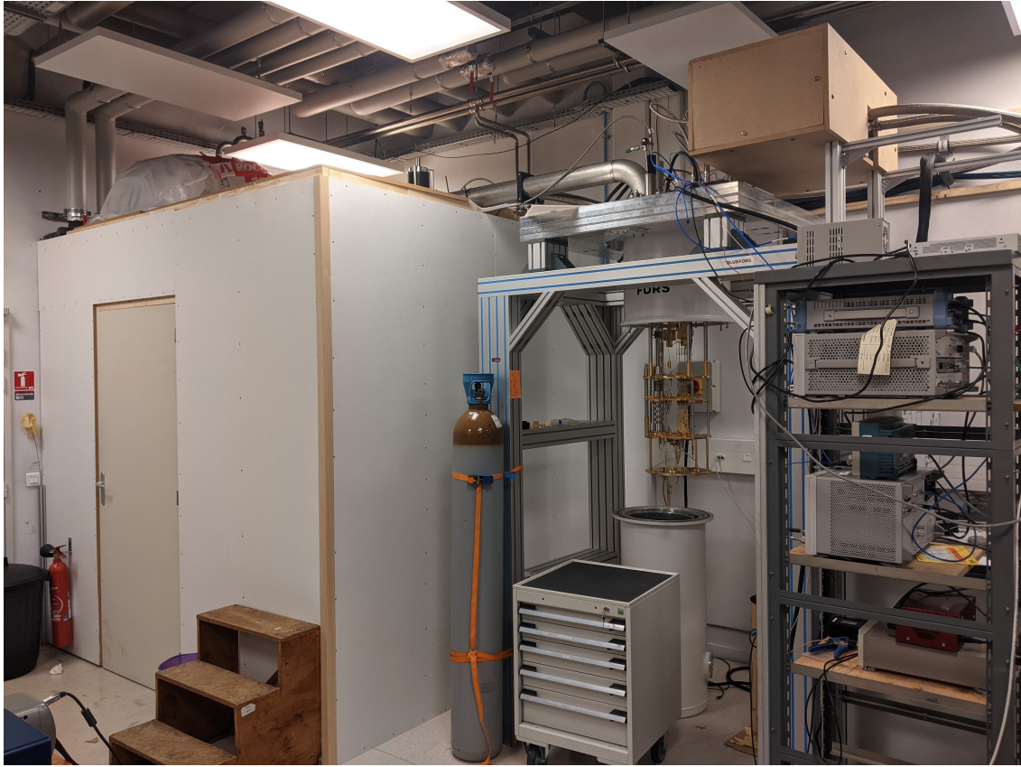
Fig. V.2 The new LKB Bluefors cryostat. The pulse tube has been isolated by building a small cabin around it. The wooden box is also for acoustic isolation. We don't know yet if this will have any effect for the vibrations disturbing the sample, but we can already tell the difference for the acoustic vibrations disturbing the PhD students.
