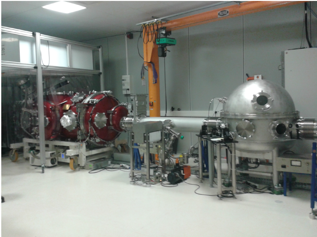
Fig. IV.33 The clean room at the CALVA facility. The red vacuum chamber (called Ferrarix) houses the in-vacuum OPO, the homodyne detection and the telescopes used to mode-match the squeezed beam to the 50-m cavity. The grey vacuum chamber houses the input mirror suspension of the rotation cavity.
