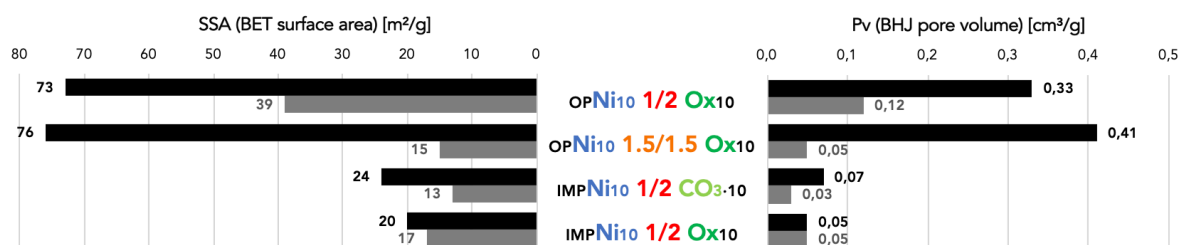
Figure 5.12: SSA and Pv for nickel catalysts pre- (in black) and post-SESR test (in grey).
