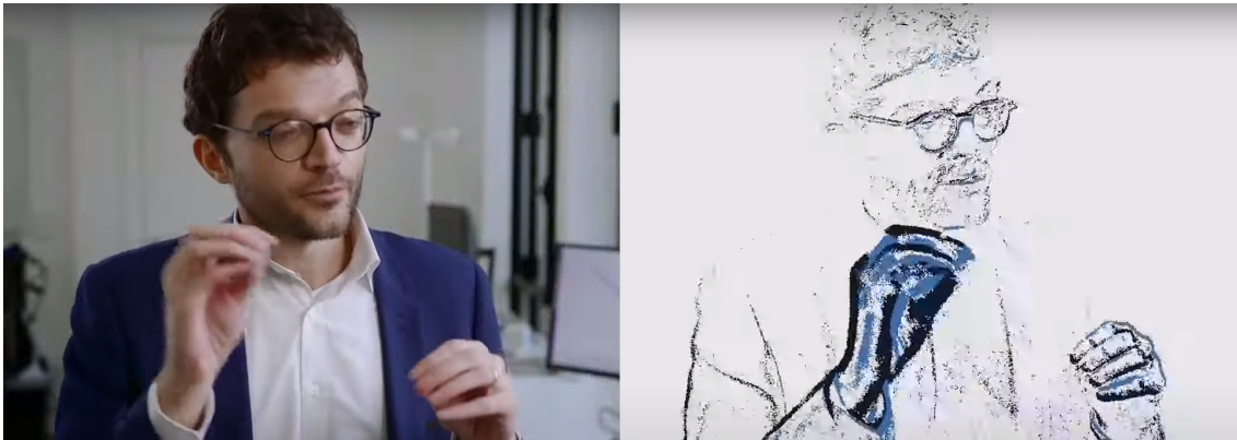
Figure 2.10: Output of an event sensor (on the right). To reconstruct this frame, events have been accumulated over a fixed time window equivalent to the duration of a single traditional frame (60ms), with blue and black events representing ON and OFF events respectively. Figure taken from (Prophesee, 2021).
