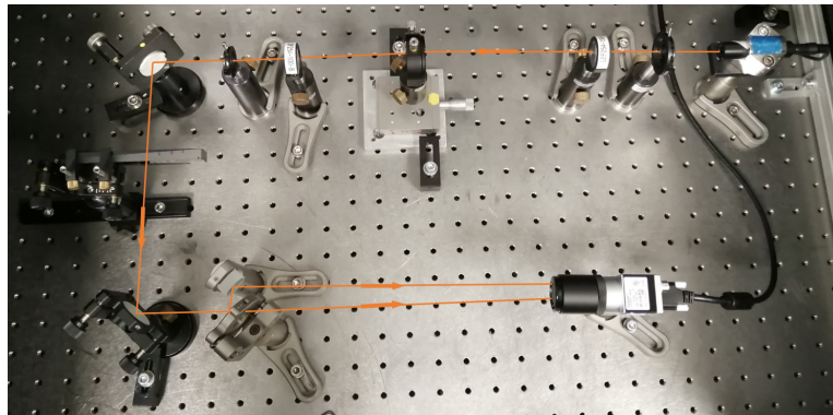
Figure 6.2: Photograph of the experimental setup to measure the spatial resolution (from figure 6.1).
