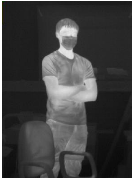
FIGURE 4.37: Image obtained using the microbolometer with a 1pt NUC. Mean of 20 images at 30 fps
