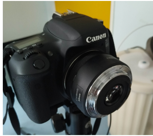
FIGURE 4.34: Close up of the reversed lens
