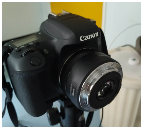
FIGURE 4.34: Close up of the reversed lens
