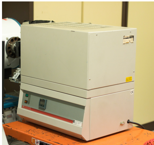
FIGURE 4.25: Cavity blackbody used for the characterization of the prototypes
