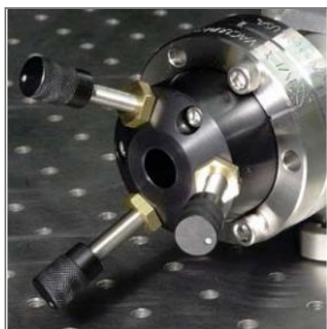
Figure 3.11 Left – cavity mirror support, LGR. Right – mirror reflectivity vs. wavelength (provided by Layertec)
