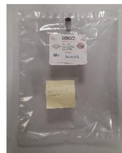
Figure 4.18 Left – schematic diagram of gas injection system used to measure the rate constant of OH in reaction with CH<sub>4</sub>. Right – photo of 4-liters gas sampling bag containing a CH<sub>4</sub>/N<sub>2</sub> mixture.
