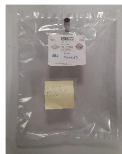
Figure 4.18 Left – schematic diagram of gas injection system used to measure the rate constant of OH in reaction with CH 4 . Right – photo of 4-liters gas sampling bag containing a CH 4 /N 2 mixture.
