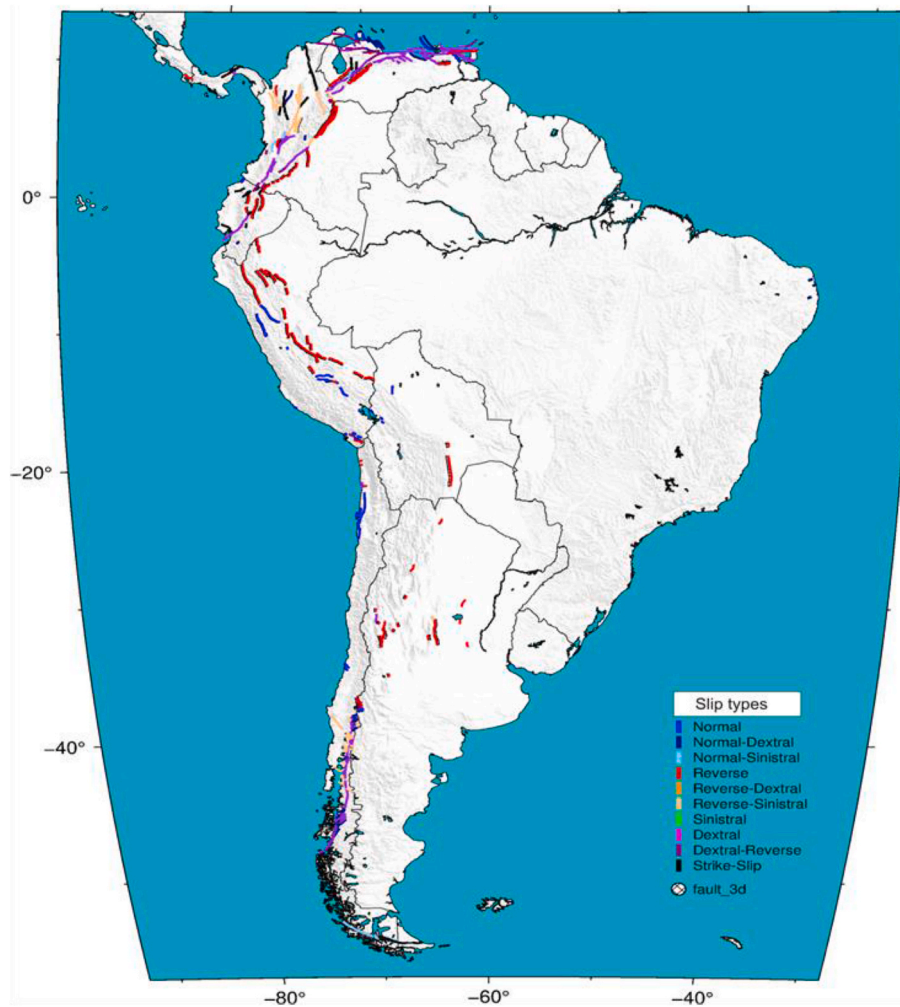
Fig. 12. Slip types of hazardous faults in Northern South America.
