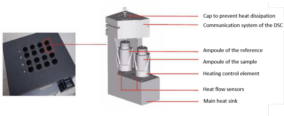
Figure 2.24: Adapted explanatory scheme of the TAM AIR microcalorimeter [Kaci, 2021]
