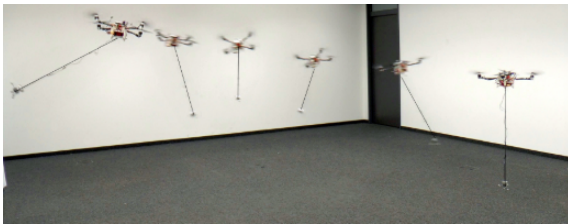
(f) Agile quadrotor manoeuvres with a cable-suspended payload [Foehn, 2017]
