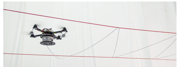
(g) Quadrotor assembling tensile structures [Augugliaro, 2013]
