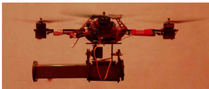
(d) Quadrotor equipped with impactive and ingressive gripper for grasping and transporting bar structures and pieces of wood [Mellinger, 2011b]
