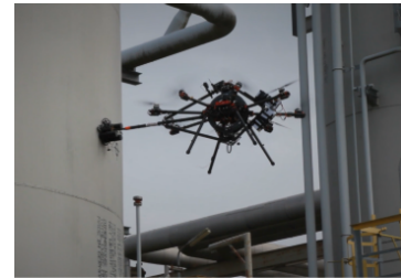
(c) AeroX: an eight-tilted rotor platform with an 6-DoF robotic arm for contact inspection [Trujillo, 2019]
