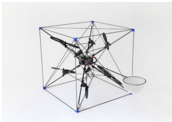
(d) A tilted octocopter with a pouch mounted to catch ball [Brescianini, 2018]
