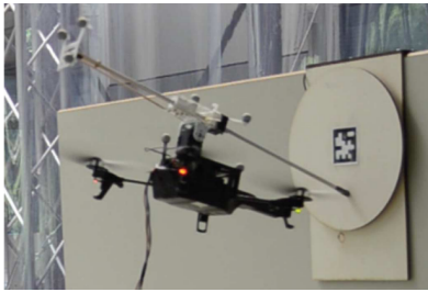
(a) Quadrotor attached with an actuated rigid link for contact-based inspection task [Bartelds, 2016]
