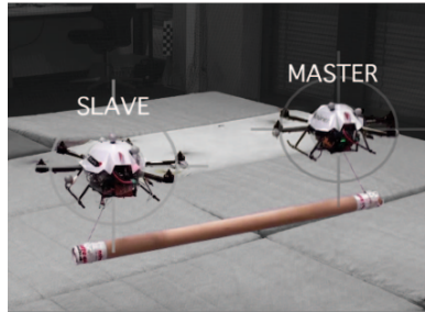
(e) Collaborative transportation of beam-like objects suspended by cables using two hexarotors [Tagliabue, 2017]
