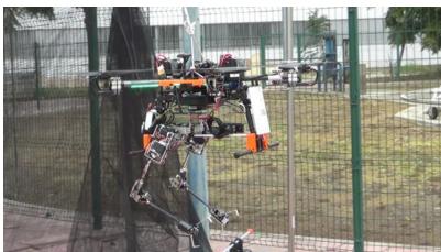
(k) Hexarotor equipped with a dual-arm system for grasping bar-like objects [Suarez, 2017a]
