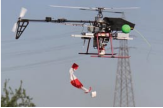
(a) Helicopter for autonomous load transportation and deployment [Bernard, 2011]
