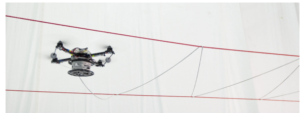
(g) Quadrotor assembling tensile structures [Augugliaro, 2013]
