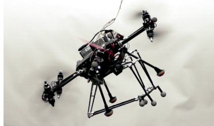
(e) An omnidirectional hexacopter with a parallel arm for pick-and-place operation [Bodie, 2021b]
