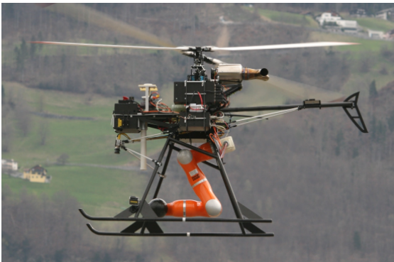
(c) Helicopter equipped with a KUKA LWR industrial manipulator [Laiacker, 2016]
