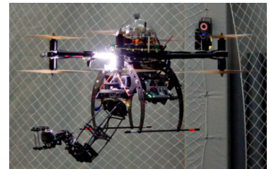
(j) Quadrotor endowed with a 6-DoF robotic arm for assembly task [Ruggiero, 2015a]
