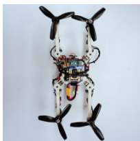
(g) A morphing quadrotor capable of folding and squeezing [Falanga, 2019]
