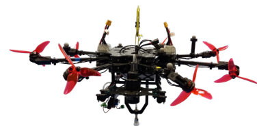
(f) dextAIR: an omnidirectional octocopter with elastic suspension [Perozo, 2022]
