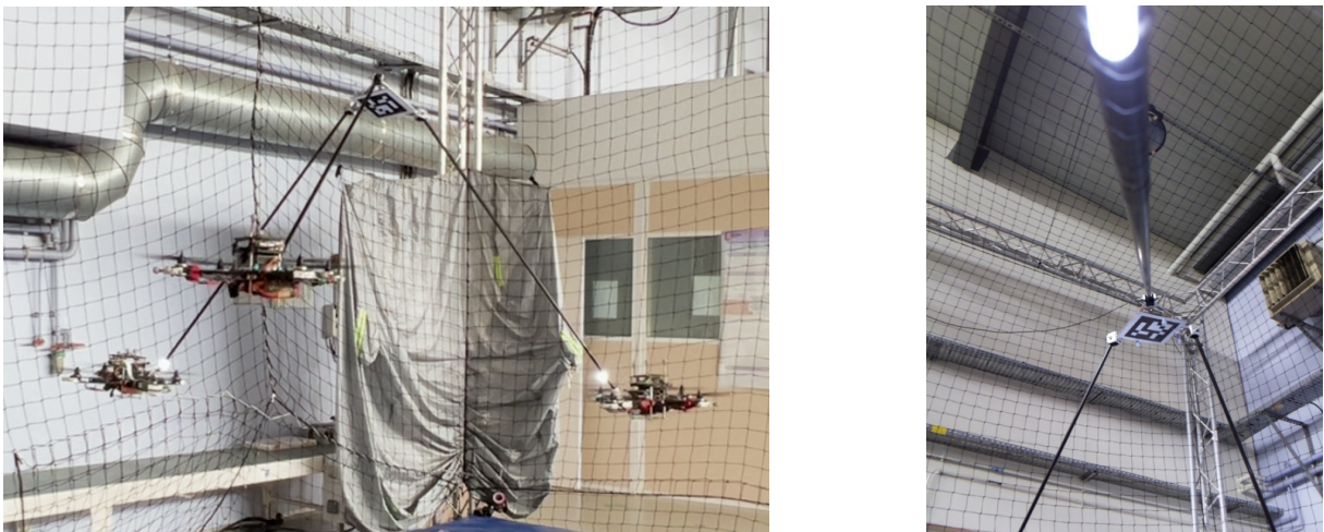
Figure 4.18 – Unfavourable configuration with large platform angle for onboard detection of the ArUco marker. Right figure shows the image captured on UAV 3 on which the marker tracking is lost.
