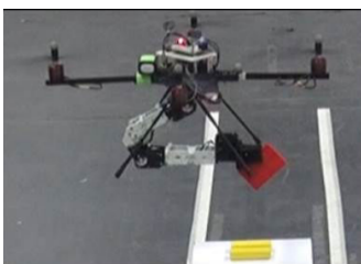
(h) Quadrotor with a 2-DoF arm for object manipulation [Kim, 2013]
