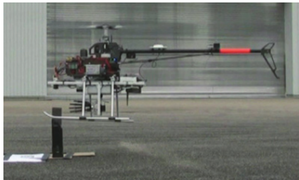
(d) Helicopter equipped with a robotic arm for grasping and manipulation [Kondak, 2013]
