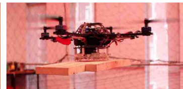
(d) Quadrotor equipped with impactive and ingressive gripper for grasping and transporting bar structures and pieces of wood [Mellinger, 2011b]
