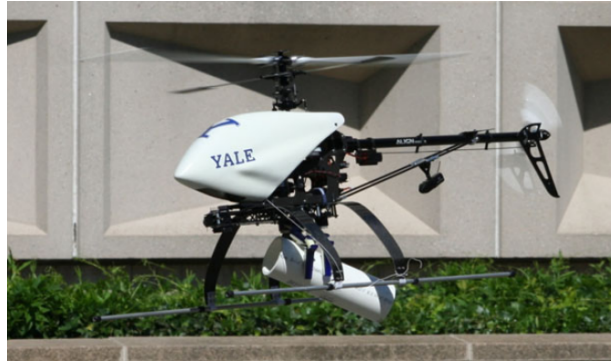
(b) Helicopter with a gripper for grasping and transporting objects [Pounds, 2012]
