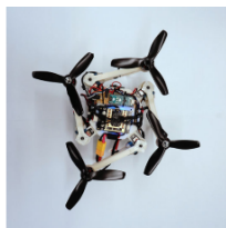
(g) A morphing quadrotor capable of folding and squeezing [Falanga, 2019]
