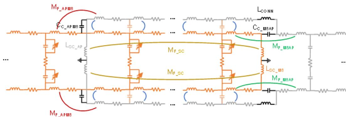
Figure 87 – Equivalent model of region 4, which shows the parasitic electromagnetic couplings between primary (in orange) and secondary (in light grey) as well as interconnection parasitics and the short-circuit terminations of both primary and secondary. Source: author.
