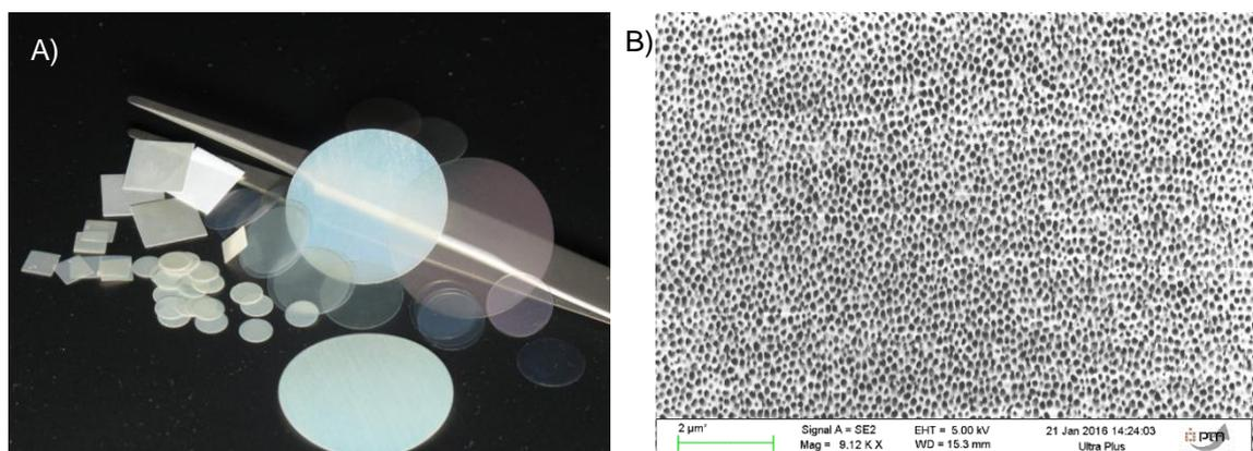
Figure 4 – A) AAO membranes in different diameters, thicknesses and pore diameters. B) Electron scan of a membrane showing the nanopores. Source: <https://www.inredox.com/products/nanofab-toolbox/aa0-wafers-packs/> and author.
