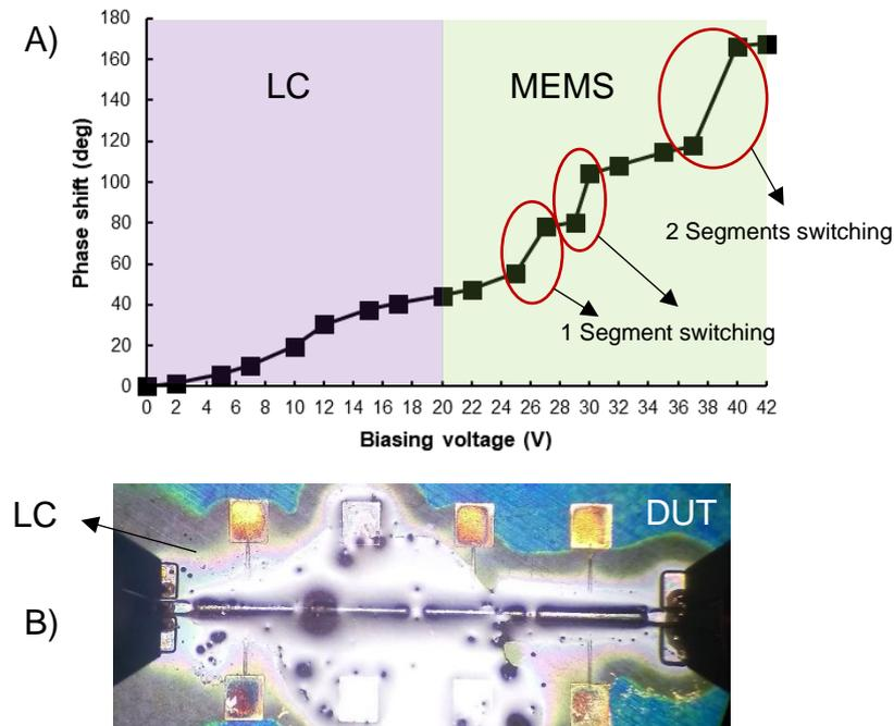
Figure 20 – a) Phase shift against biasing voltage of a device having  $L_S = 500 \text{ um}$ ,  $N_S = 4$  and  $W_S = 25 \text{ um}$  showing clearly the two different regions of operation of the LC MnM phase shifter. b) Device under test showing the liquid crystal injected under the device. Source: author.
