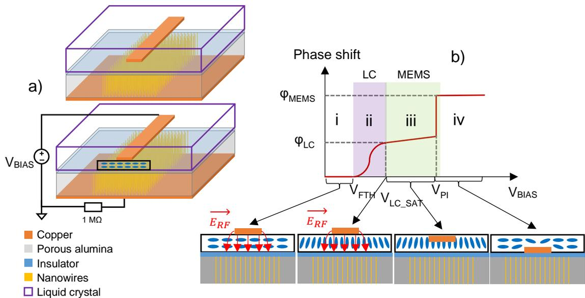
Figure 16 – a) A side view of the LC-MnM phase shifter showing the main elements and the biasing scheme to bias the liquid crystal and to create electrostatic switching. b) Phase shift of the LC-MnM phase shifter as a function of the applied bias voltage, showing in detail the signal strip position and the liquid crystal orientation in each region. Source: author.
