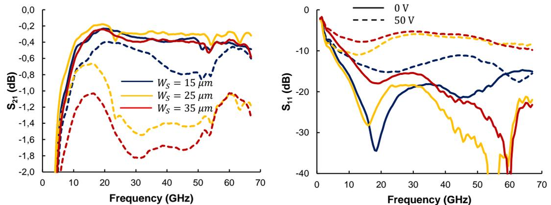
Figure 27 – Insertion loss (left) and return loss (right) for three different, single-segment LC-MnM MEMS phase shifters at zero bias and at  $V_{BIAS} = 50$  V, larger than  $V_{PI}$  for all devices. Source: author.
