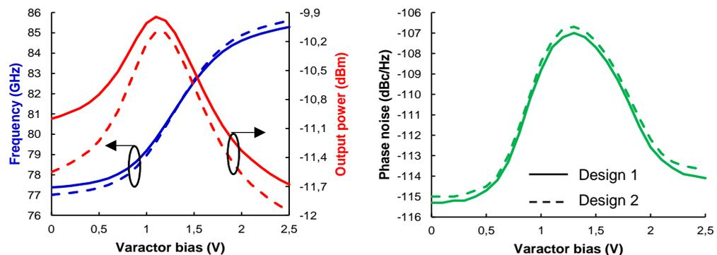
Figure 53 - Post-layout simulation results containing the output frequency (in blue), the output power (in red) and the phase noise (in green) for the two proposed tank designs. Source: author.
