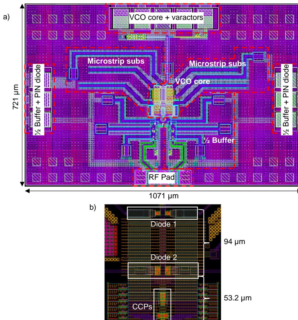
Figure 95 – a) Final layout of the multiband VCO, including the RF chokes for the two RF switches, the output buffers, the DC biasing pads and the RF pads. The die dimensions are also shown. b) The tunable S-CPS transformer-based resonator is shown in detail, with the primary and secondary lengths. Source: author.
