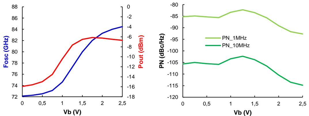
Figure 76 - Post-layout simulation results of the distributed, tapered CCP VCO, showing the output frequency (blue) and power (red), as well as the phase noise at 1 MHz offset (light green) and at 10 MHz (dark green). Source: author.
