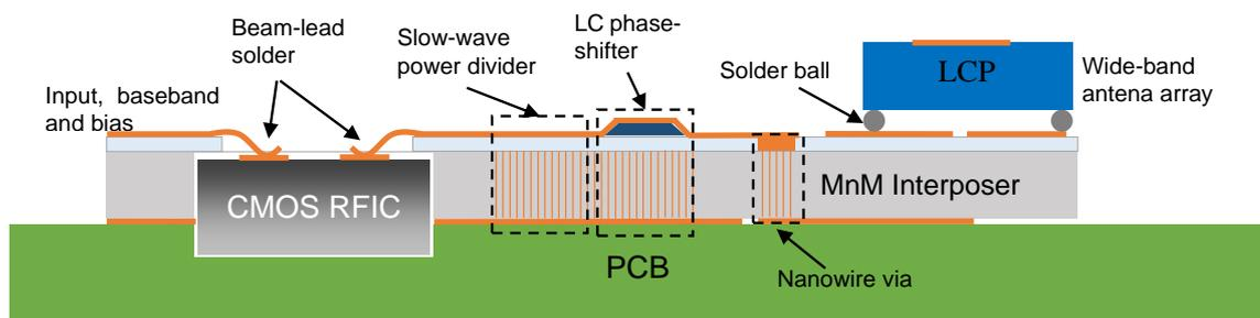
Figure 3 - Cross-section of a MnM-based mmW front-end, showing several devices and integration techniques to realize it. Source: author.
