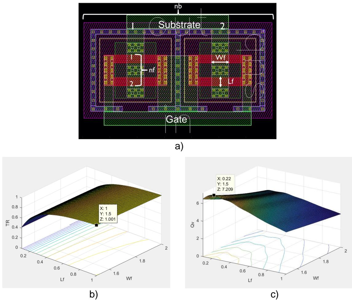
Figure 39 - a) PCell varactor layout with the design variables highlighted. b) Tuning range and c) zero-bias quality factor for thick-oxide PCell varactors for  $100 \text{ nm} < L_f < 1 \text{ }\mu\text{m}$  and  $1.5 \text{ }\mu\text{m} < W_f < 2 \text{ }\mu\text{m}$ . Source: author.
