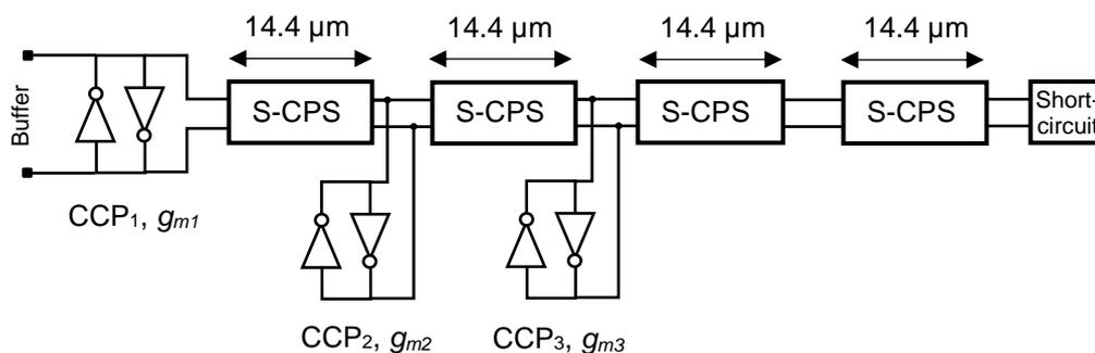
Figure 74 - Schematic representation of the distributed CCP VCO. Source: author
