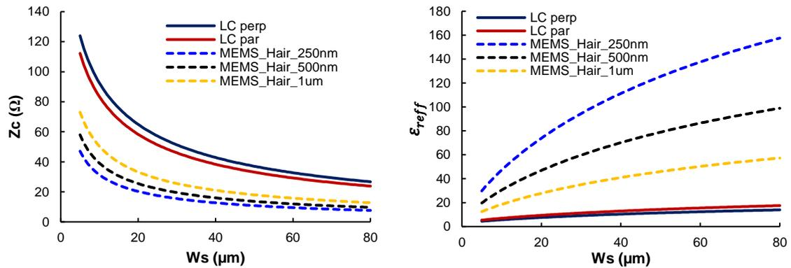
Figure 19 – Characteristic impedance and effective dielectric constant of the suspended segments of the LC-MnM phase shifter, obtained from the equivalent model of the suspended microstrip line with the addition of the liquid crystal effects. Source: author.
