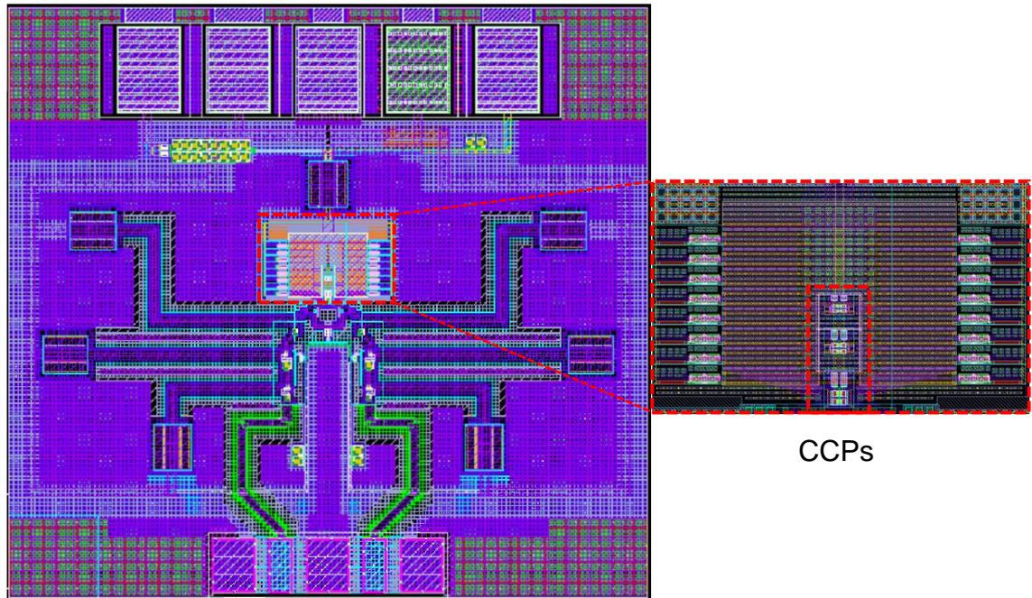
Figure 75 - Distributed CCP VCO layout plus the tank in detail. Source: author.
