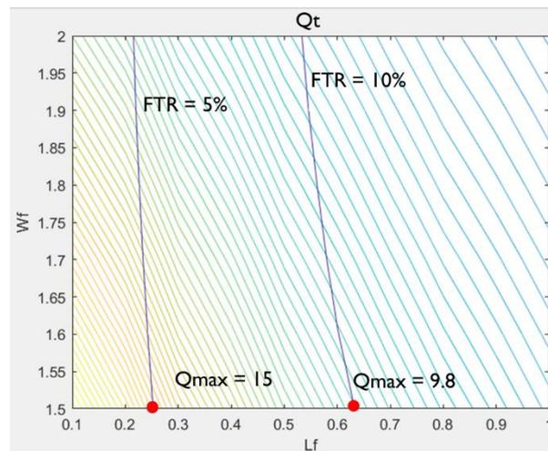
Figure 58 – The Q-factor level curves for a mock resonator, showing the *loci* of  $FTR = 5\%$  and  $FTR = 10\%$  as dark blue lines. The Q-factor increases toward the lower left corner of the graph. Source: author.
