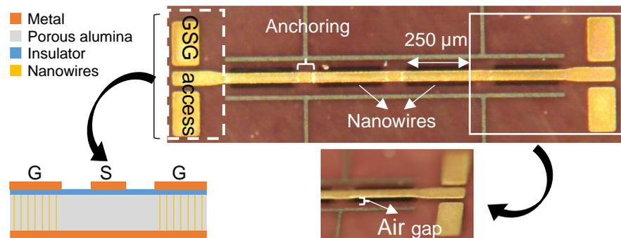
Figure 10 – Photo of a fabricated suspended microstrip line with  $W_S = 25 \mu\text{m}$ , 4 segments and  $L_S = 250 \mu\text{m}$  showing the RF pads, the regions filled with nanowires and the air gap between the substrate and the signal strip. Source: author.
