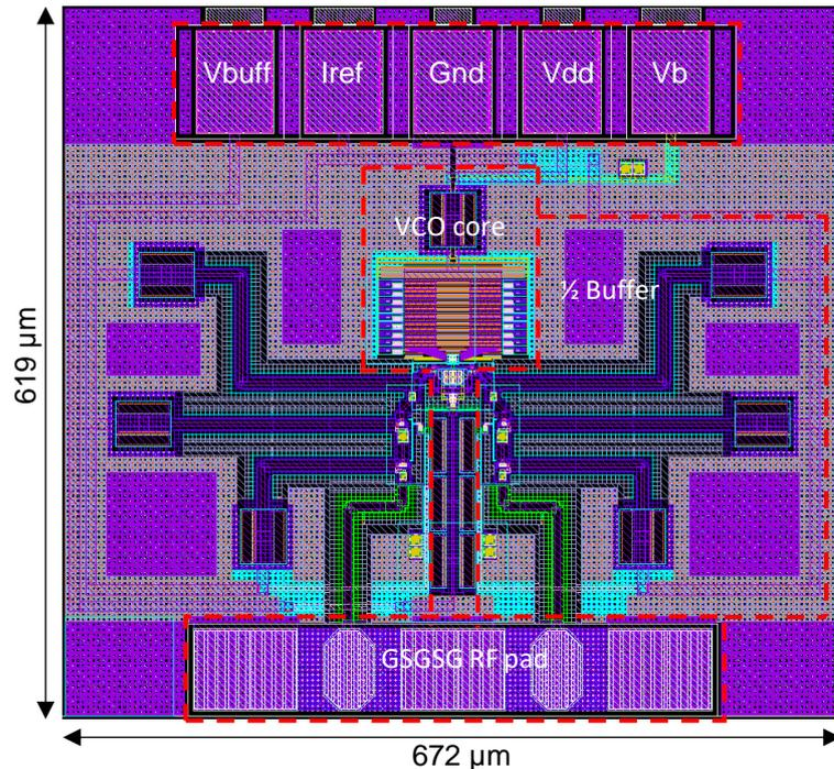
Figure 66 - Final layout for the optimized VCO at 80 GHz. Source: author.
