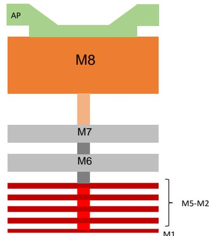
Figure 32 - The Back-end of line stack of the 55-nm BiCMOS technology, showing the metallic layers and vias. Source: author.
