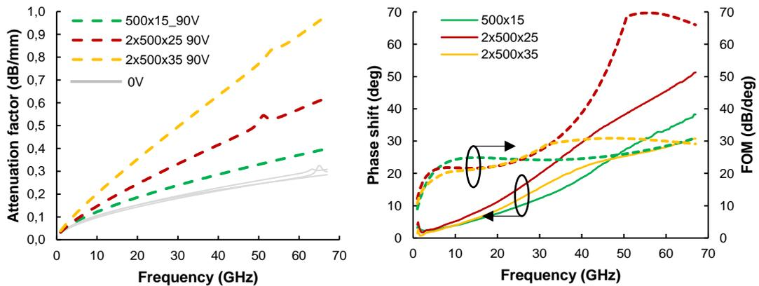
Figure 25 – Attenuation factor (left), phase shift and FOM (right) for the four suspended microstrip lines, MEMS phase shifters analyzed in this subsection. Source: author.
