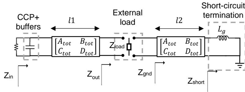
Figure 80 – Bufferless resonator model, which is based on the shifted CCP model presented in Figure 69. Source: author.
