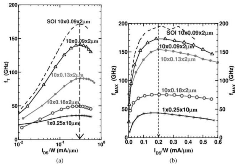
Figure 29 -  $f_t$  (a) and  $f_{max}$  (b) of n-channel MOSFETs of different CMOS technological nodes versus drain current density. The nodes are: 250 nm, 180 nm, 130 nm and 90 nm bulk processes. The 90 nm, SOI process is also included for comparison. Source: [55]
