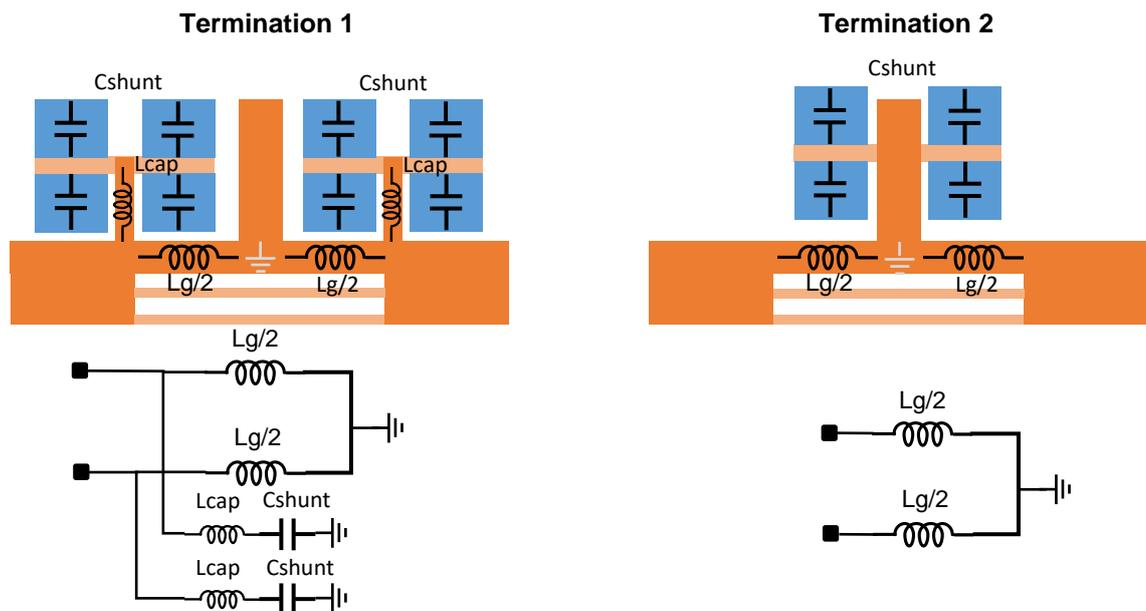
Figure 41 – Basic layout and equivalent electrical model of the two short-circuit terminations proposed for the loaded S-CPS resonator. Source: author.
