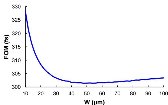
Figure 90 - Figure of merit at 80 GHz of MOSFETs for channel widths between 10  $\mu\text{m}$  and 100  $\mu\text{m}$ . Source: author.
