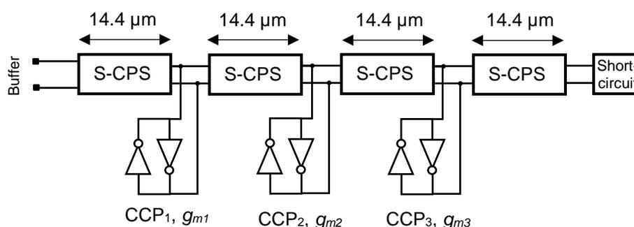
Figure 77 - Schematic representation of the shifted, distributed CCP VCO. Source: author.
