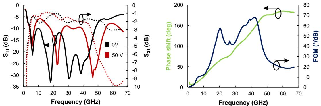
Figure 26 – Return loss and insertion loss (left), phase shift and FOM (right) for the LC-MnM MEMS phase shifter having  $W_S = 25 \mu\text{m}$ ,  $L_S = 500 \mu\text{m}$  and  $N_S = 4$ . Source: author.
