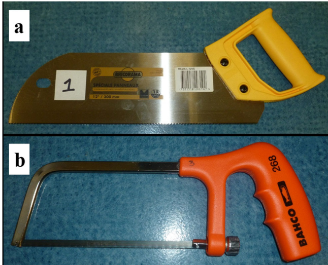
Fig. 1 Handsaws selected for this study. a Universal panel saw. b Rip hacksaw
