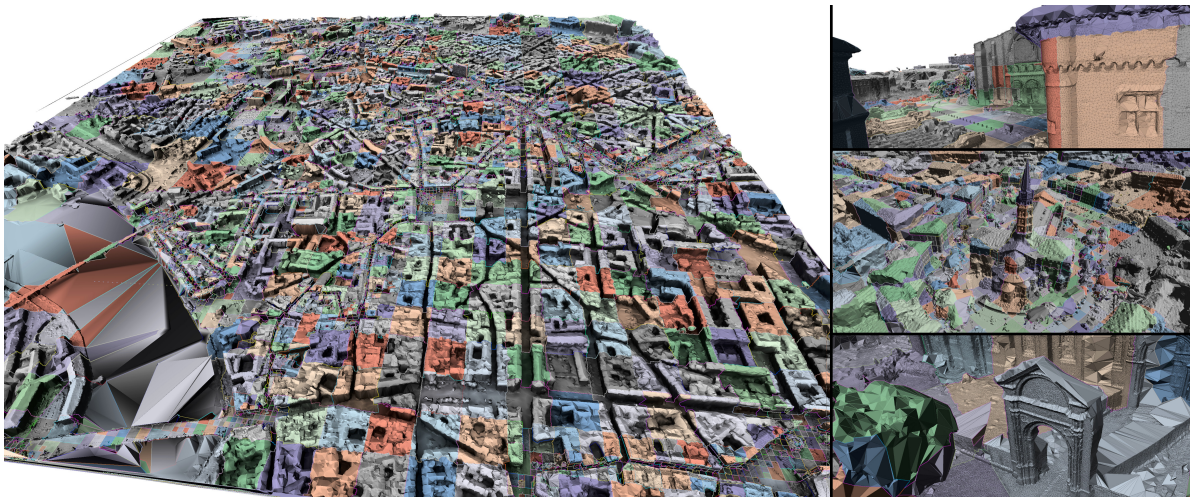
Figure 2.8: Reconstruction result on a 350 million points data set. Tiling is visualised through a random colour per tile.
