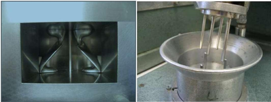
**Figure 10.** Geometry of the mixing system in Farinograph (left) and Mixograph (right). Copied from (Frédéric Auger, 2008)
